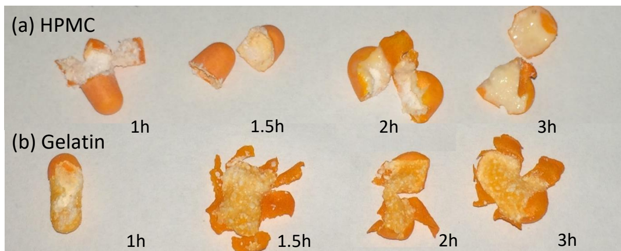
Figure 3.12 Inside of gelatin and HPMC Capsules after dissolving for different time (RS: RL=1:2; Weight gain \approx 6 \text{ mg/cm}^2 )
