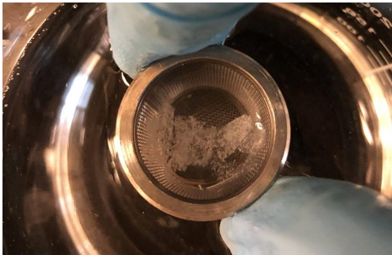
Figure 5.3 The thin film observed after dissolution test of dry powder coated tablets without sub-coating
