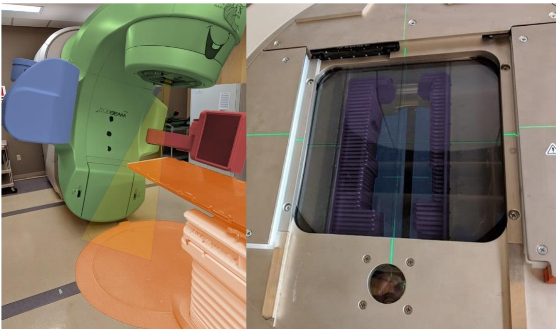
Figure 1.1: Picture of a linac [left] and the linac's treatment head (collimator) [right]. Note that these images have been recolored to help identify each component. [left] The patient lies on the treatment couch (orange) during treatment. Ionizing radiation is delivered from the gantry (green) towards the patient, as illustrated by the yellow cone. The gantry (and therefore the beam) can fully rotate around the patient, while the couch can be rotated, elevated, and repositioned as well. Some linacs possess onboard imaging capabilities for patient positioning and setup. The x-ray source and detector of this linac's imaging unit is highlighted blue and red, respectively. [right] The beam can be attenuated and shaped using the jaws (blue) and the multileaf collimator (MLC, purple) within the collimator of the linac. The rotation angle of the collimator can also be adjusted.
