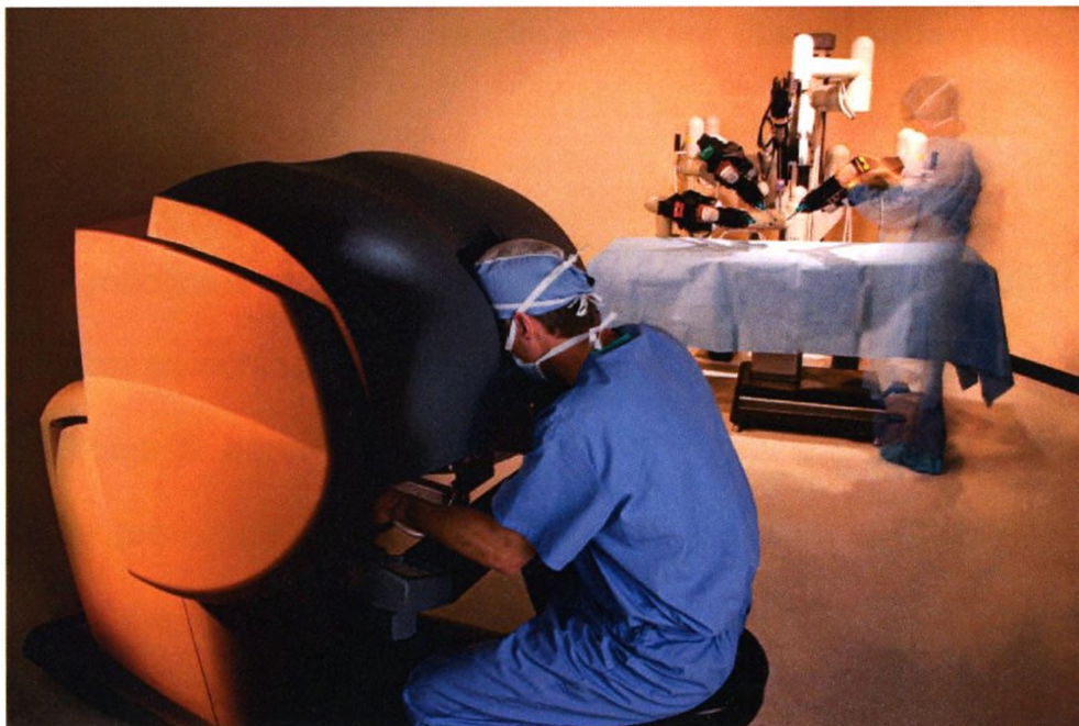
Figure 1. The da Vinci surgical system. The surgeon controls robotic instruments while sitting at a console in an unsterile area of the operating room. A bedside surgeon and scrub nurse assist with external arm adjustments, instruments changes, or port placement changes. (Source: Media courtesy of Intuitive Surgical Inc.).
