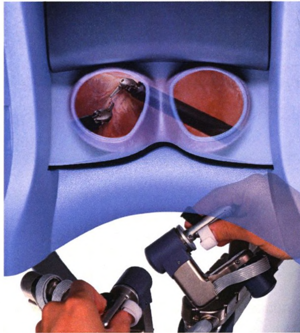
Figure 2. The surgeon operates while viewing a three dimensional image of the surgical site at the console. The thumb and index finger are used to control the robotic instruments. Each robotic instrument has seven degrees of freedom motion – three translational planes plus pitch, yaw, roll and open/close at the end effector. (Source: Media courtesy of Intuitive Surgical Inc.).
