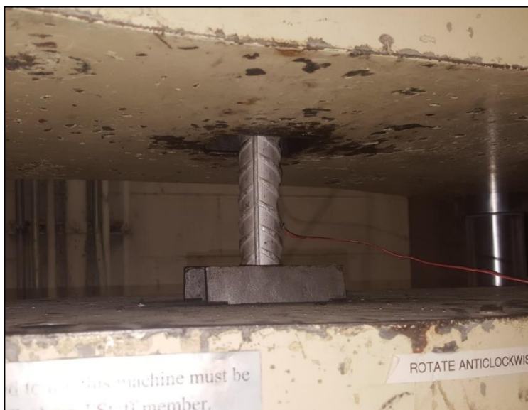
(a) Steel bar during testing
