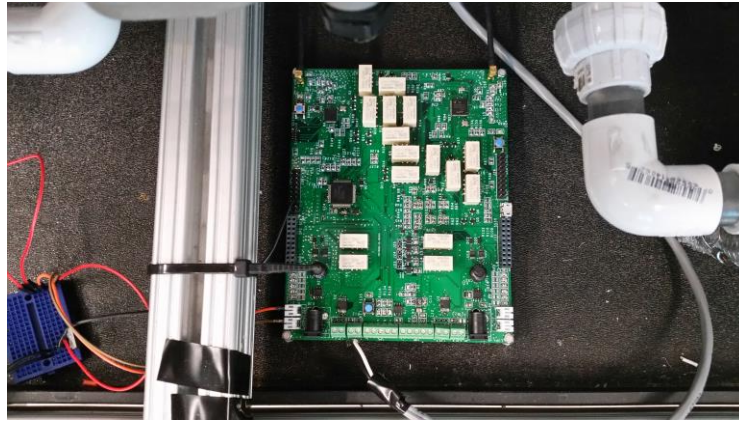
Figure 6.7: A one-module device interfaced to the NPCTF.
