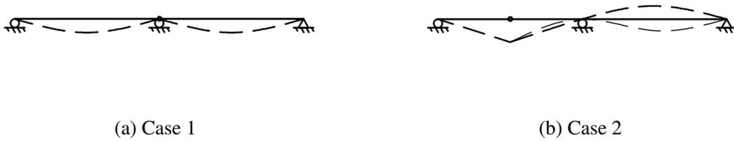
Figure B.3: Elastic curves for two-span beams
