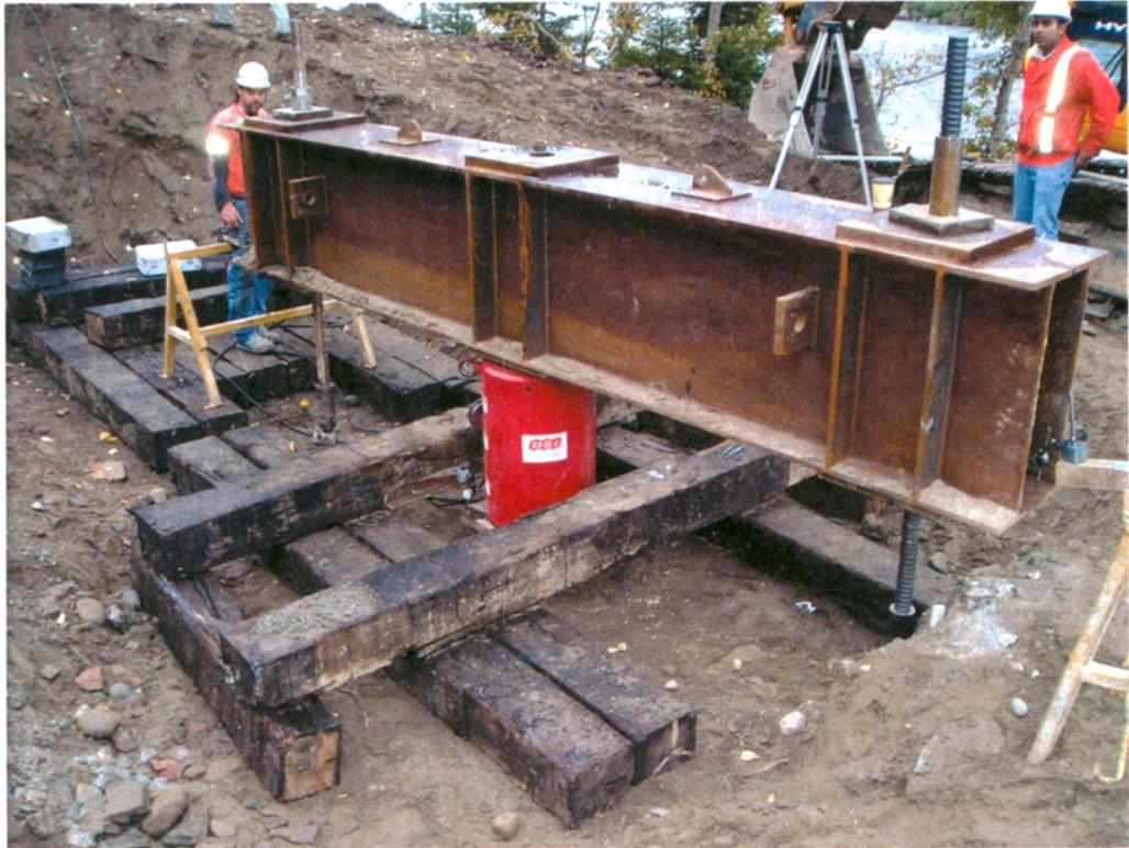
**Figure 3.7** Typical Micropile Compression Test Set Up. (Note: The timbers were used temporarily to support the reaction beam prior to jacking)
