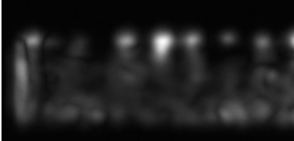
Figure 6. US C-scan image obtained from scanning with 2.25MHz transducers and through transmission method in acoustic microscope.
