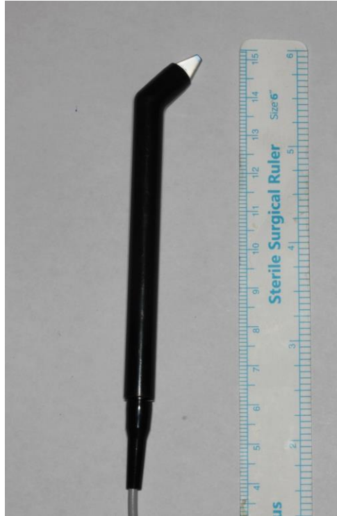
Figure 11. Intra-oral US device with ruler for size comparison.
