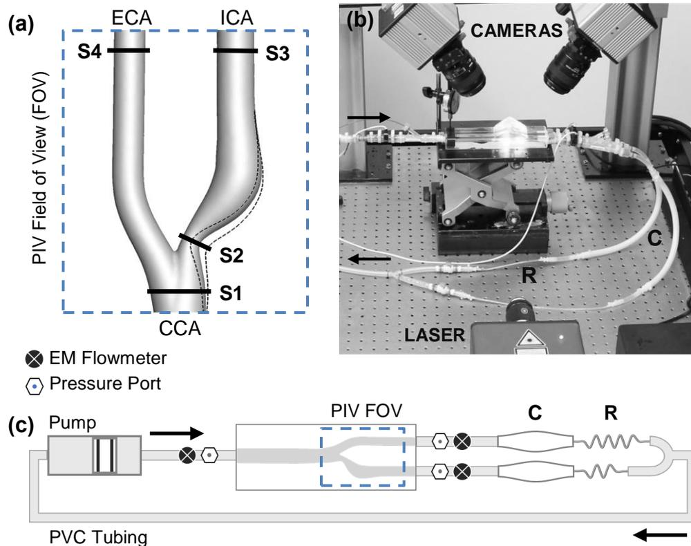
**Figure 3.1:** a) Phantom geometry with 50% eccentric stenosis. Dashed lines indicate the boundaries of 30% and 70% stenosed geometries. CCA: common carotid artery, ICA: internal carotid artery, ECA: external carotid artery; b) Photo of the experimental setup. Arrows indicate flow direction from and to pump; c) Schematic diagram of flow circuit (not to scale) including compliant (C) and resistive (R) elements. Direction of flow indicated by arrows.
