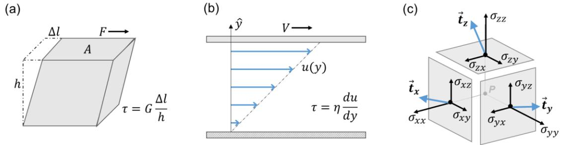
**Figure 1.1:** (a) A shear stress applied to an elastic material is related to the deformation by the elastic modulus,  $G$ . (b) In a simple shear flow, the shear stress on the fluid is related to the rate of deformation. (c) The elements of the stress tensor in three dimensions acting on a fluid element at point  $P$ .
