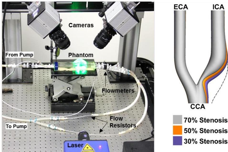
**Figure 2.1: Experimental set-up including flow circuit and PIV components (left). Family of carotid artery bifurcation geometries with progressing degrees of eccentric stenosis (right). Dashed contour line indicates the boundary of the normal, disease-free geometry. CCA: common carotid artery, ICA: internal carotid artery, ECA: external carotid artery**
