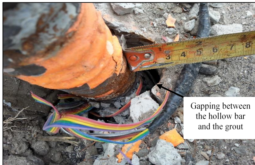
Figure 5-8 Local failure mechanism due to cyclic loading
