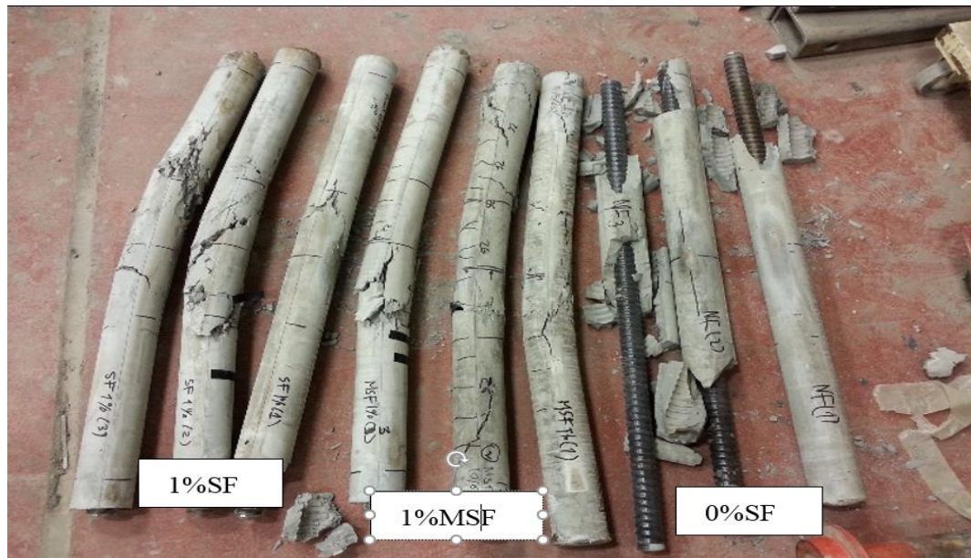
Figure 6-6 Post cracking behaviour of fiber reinforced and non-reinforced grouted micropiles
