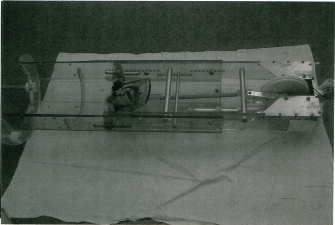
**Figure 2.** Custom-built MR-compatible ankle exercise ergometer used during the experimental protocol.
