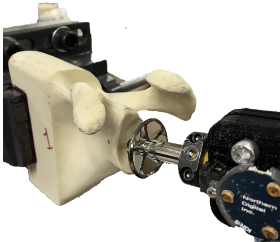
Figure 4-3 Arrangement of the reamer against the Sawbone scapula model in pre-start position.
