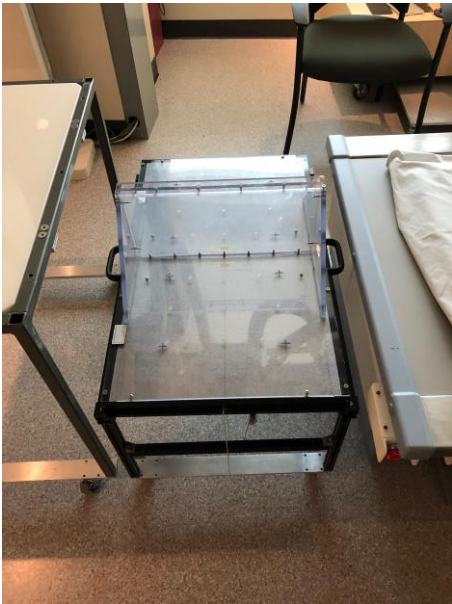
Figure 2.4 Fiducial bead marker cage
