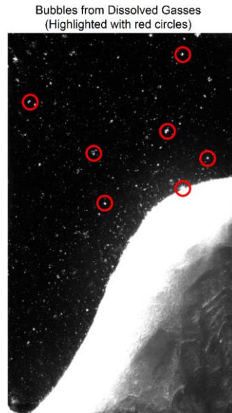
Figure 8: Highlighted bubbles from dissolved gasses during lauric acid melting
