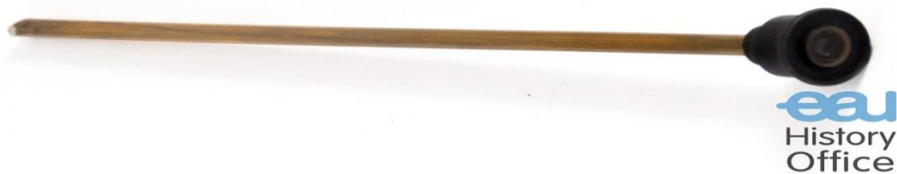
Figure 2: Optical tube after Max Nitze. Courtesy of the History office at the European Association of Urology. From the Int. Nitze-Leiter Research Society for Endoscopy, Vienna/Reuter Collection. http://history.uroweb.org/history-of-urology/diagnosis/looking-into-the-body/nitze-cystoscope/
