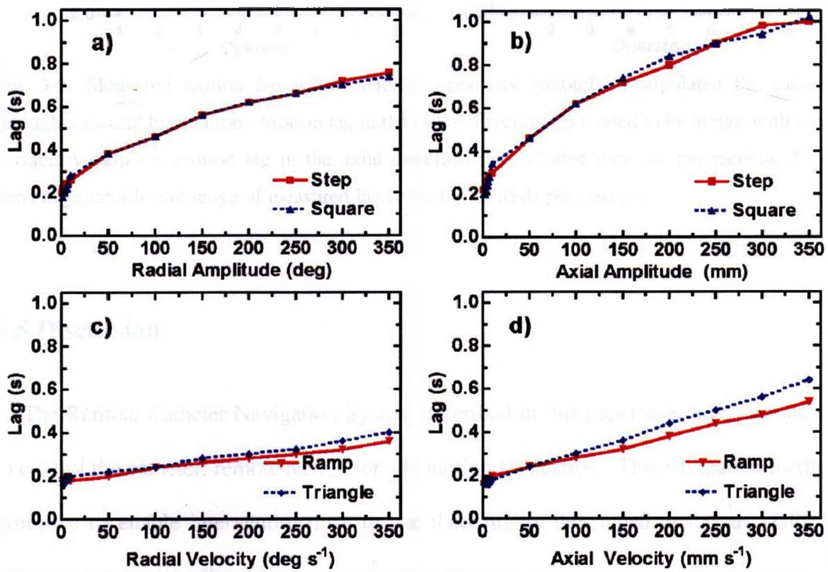
Fig. 3-4: Measured replicated motion lag time using known motion profiles: a) step/square response in the radial direction, b) step/square response in the axial direction, c) ramp/triangle response in the radial direction, and d) ramp/triangle response in the axial direction.
