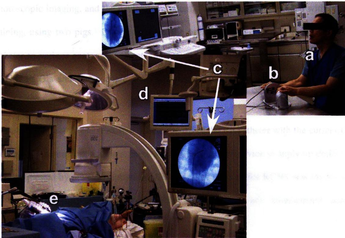
Fig. 5-1: The RCNS integrated into an experimental procedure suite. The operator (a), situated approximately 3 meters from the patient bed, manipulates the input catheter inside the CS (b) while viewing the 2D fluoroscopic images (c), and the ECG (d). Mounted on an articulated arm, the CM (e) replicates the motion of the input catheter, inside the pig. The workstation of the RCNS is placed beside the operator (not shown).
