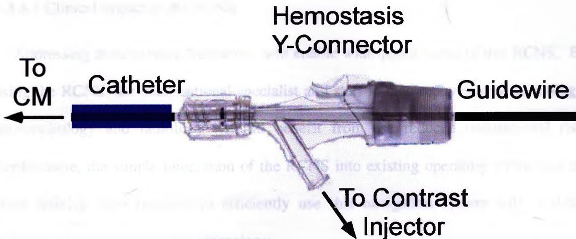
Fig. 6-2: A hemostasis connector placed at the proximal end of a catheter during remote vascular angiography. Once the guidewire is withdrawn, an o-ring (not shown) placed inside the connector stops bleeding through the catheter. A mechanical contrast injector can be connected to the open connector for remote contrast injection.
