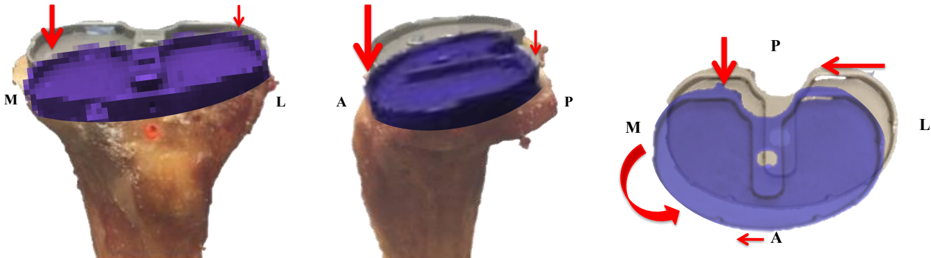
Figure 4.2. Schematic representation of primary TKA post-cycle micromotion.
