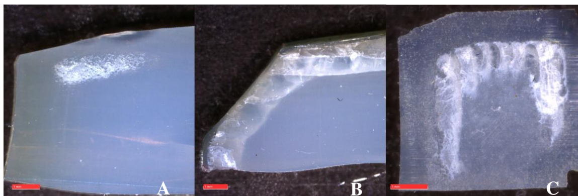
Figure 6-6 - Representative optical images of oxidized liner rim cross sections. (A) Remelted liner rim with OI_{max}=1.89 and in vivo time of 7.93 years. (B) Single annealed liner rim with OI_{max}=5.57 and in vivo time of 13.4 years. (C) Sequentially annealed liner rim with OI_{max}=3.96 and in vivo time of 6.79 years
