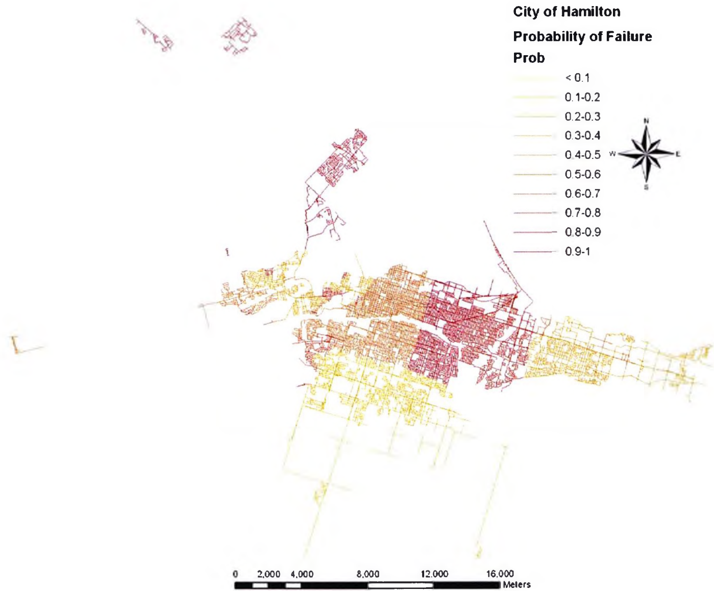
Figure 3.19 Calculated failure probability P(\tau) according to Eq. (2.11)
