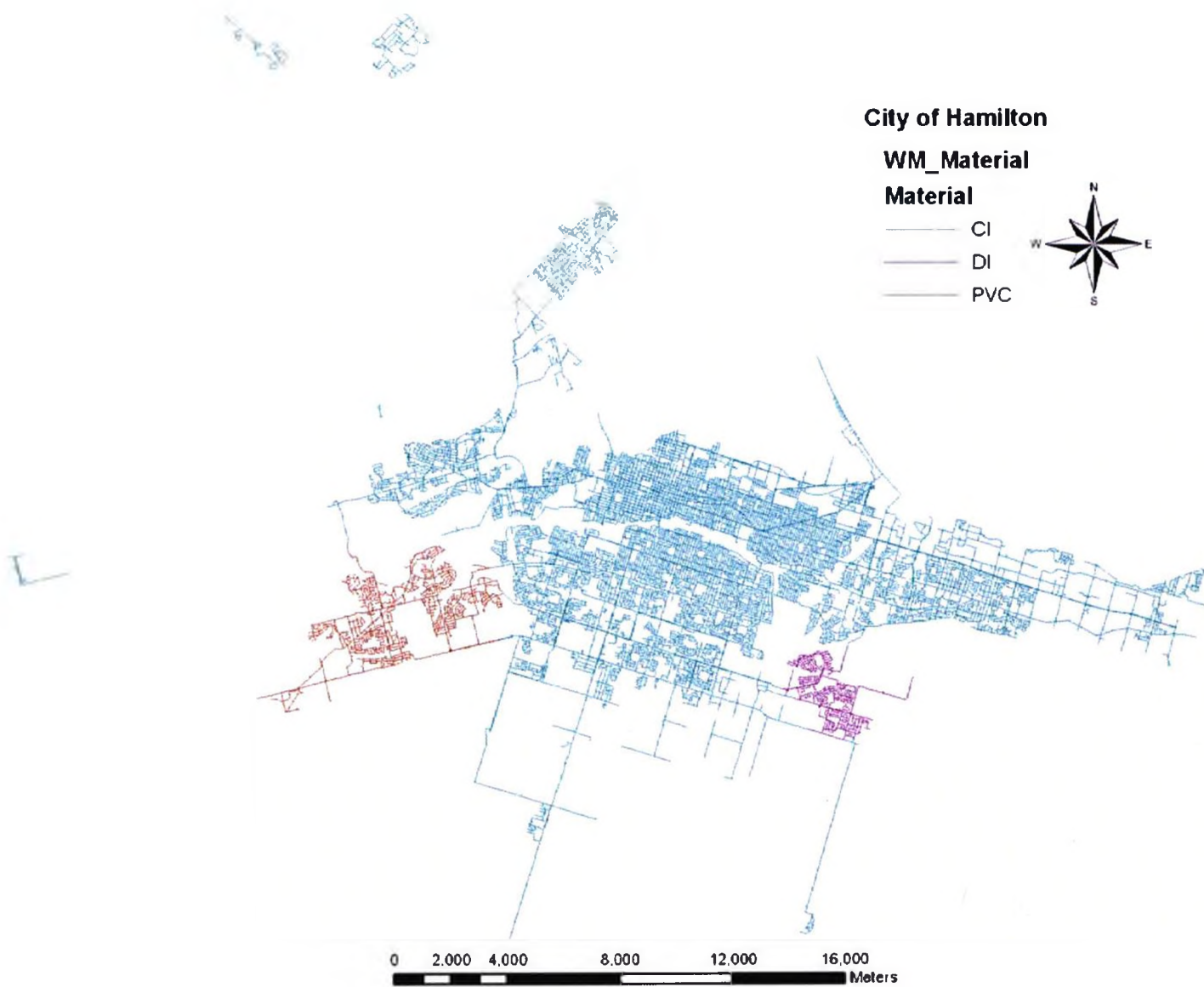
Figure 3.4b Hypothetical information on pipe materials.
