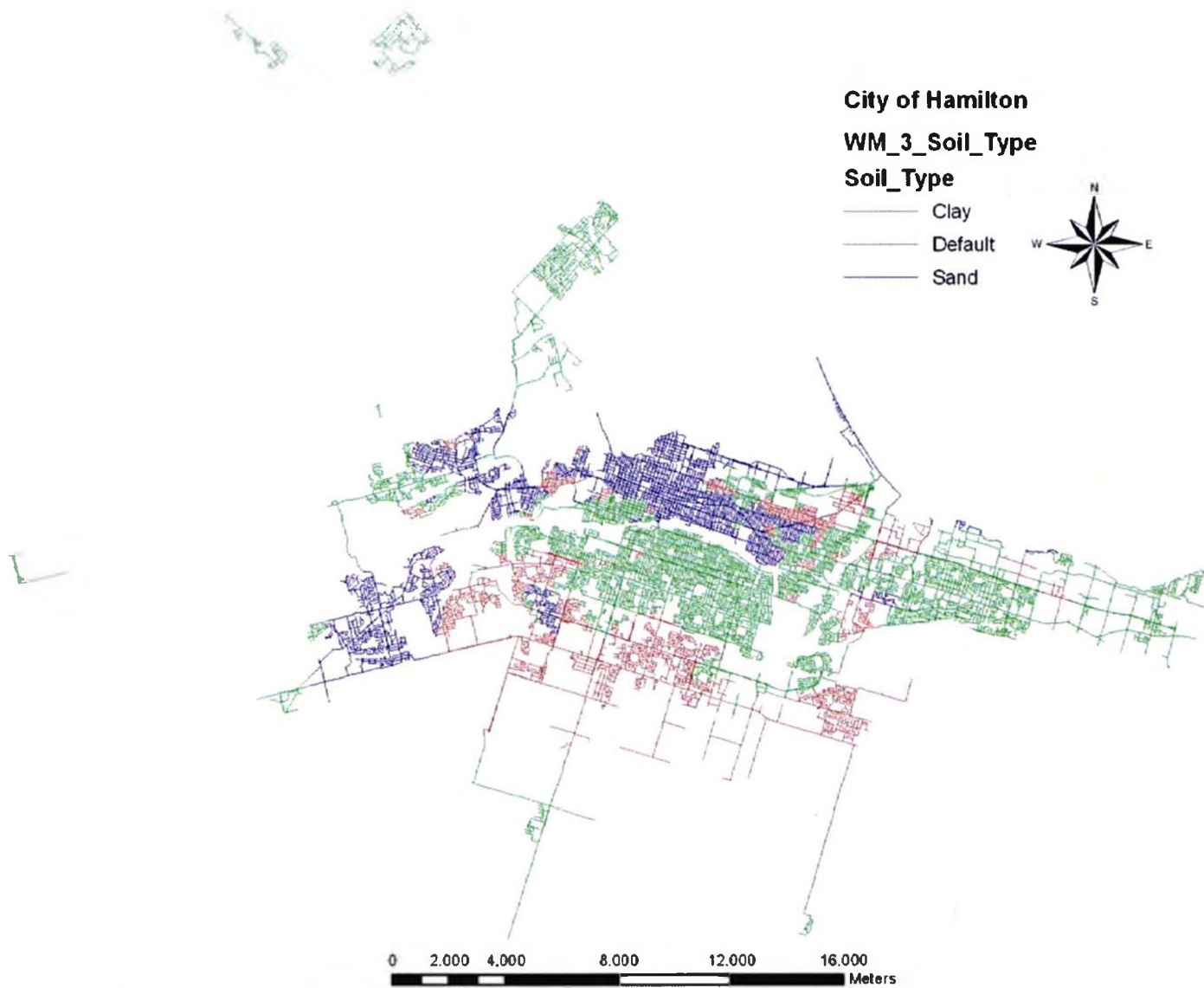
Figure 3.6b Intersection of the water main network feature layer and the 3 simplified “soil type” feature layer.
