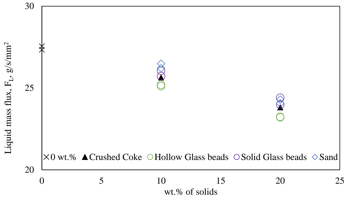
Figure 3.1: Impact of slurry concentration on liquid mass flux (water) at 2 wt.%
