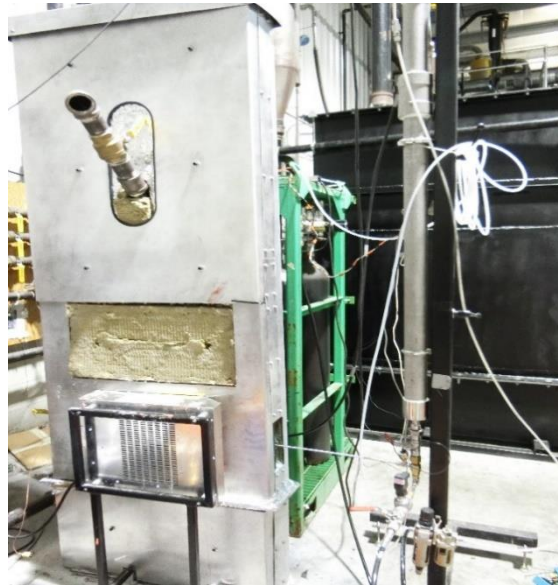
Figure 2.12: Photo of fluidized bed system
