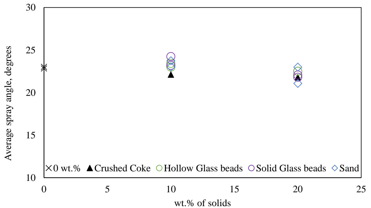
Figure 3.8: Average spray Angle vs wt.% of solids
