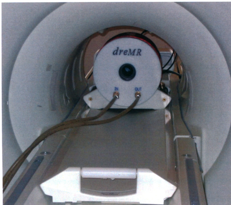
Figure 4.1. The dreMR electromagnetic insert rests upon the patient bed of an MRI machine. In this image, the cooling lines are visible.
