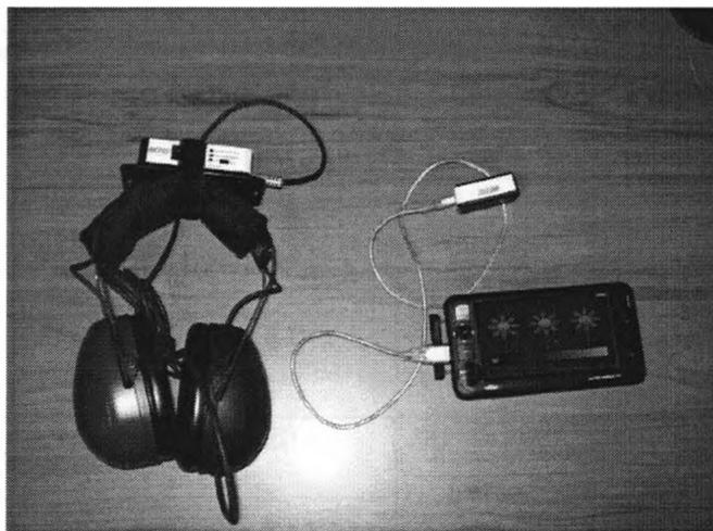
**Figure 5-2 Headphones with Receiver and a Handheld PC Running Psychoacoustic Test Software**
