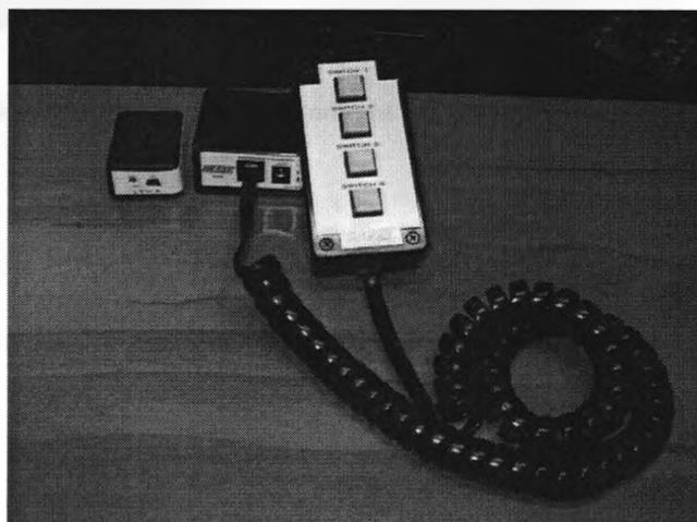
Figure 5-1 Wireless Transmitter and Receiver with Response Buttons
