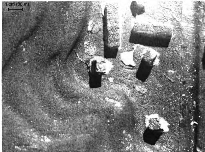
Figure 2.10: The region of interest in the horizontal plane measurements for the valley. The dimensions of the region of interest are  $15\text{cm} \times 11.3\text{cm}$ . The length scale is also provided for the model scale and full-scale (in parenthesis). The free-stream flow is from top to bottom of the image.
