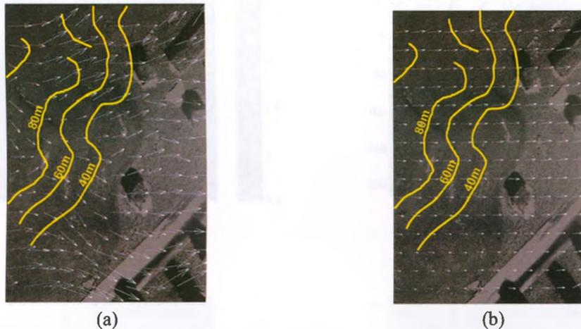
Figure 2.27: Velocity vectors for the ridge flow in a horizontal plane at  $z = 255\text{m}$ . (a) Instantaneous velocity field, (b) Mean velocity field. The velocity vectors are superimposed on the topography image.
