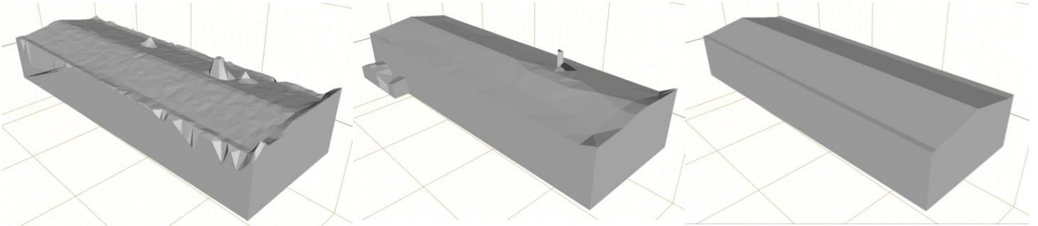
Figure 5-1: Examples of models of the same building produced by the ENVI+TIN (left) and Dual Contouring (centre) methods from original density ( $n=1$ ) LiDAR data are shown with the reference model (right) of the same building.
