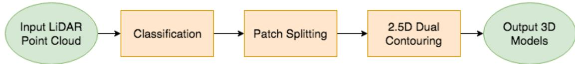
Figure 4-7: A simplified diagram of the 2.5D dual contouring pipeline.
