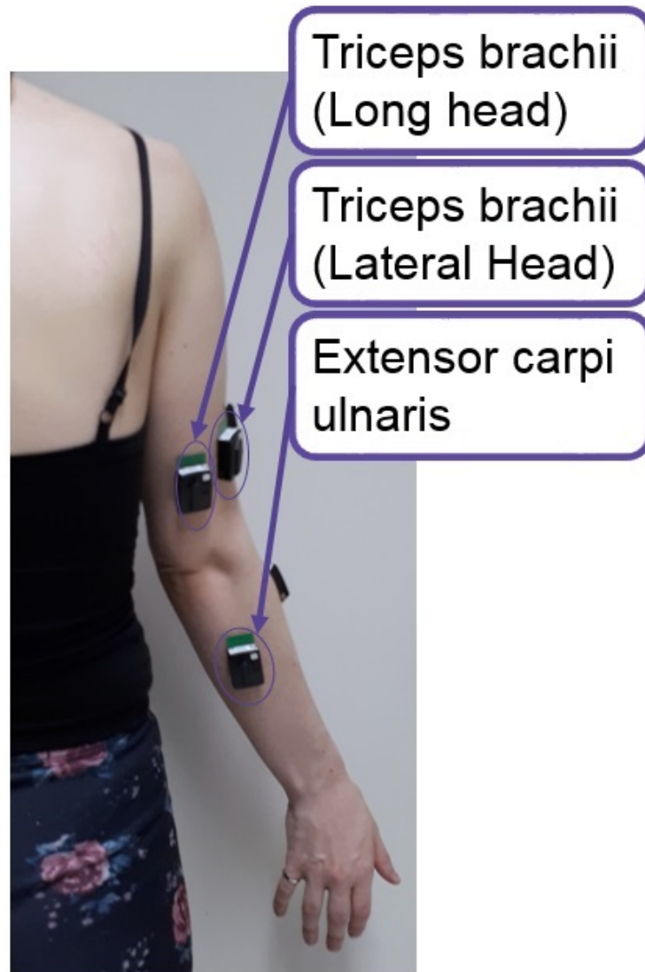
Figure 3.7: sEMG sensor placement (posterior view).
