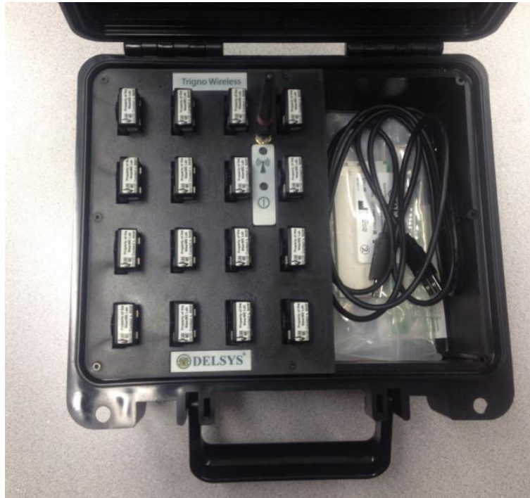
Figure 3.1: Trigno base station for charging and RF communication with sEMG sensors.
