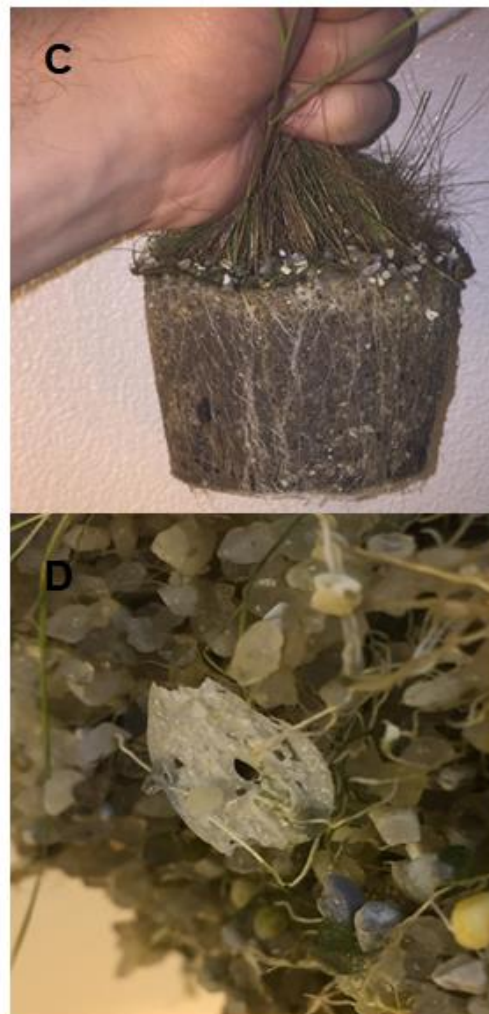
Figure 3-5 Mass loss profiles for coatings imbedded in pots with either creeping bentgrass roots, gravel substrate alone, or weekly dosages of pH 5 0.1M citrate buffer at 22 °C or 30 °C: A) PEtG:PCL; B) PEtG:PLA; C) Representative image of root bound creeping bentgrass; D) Roots imbedding into a PEtG:PCL coating. Pots were stored in growth chambers with 16 h of light, and 8 hours of darkness under 70% humidity. Dotted lines represent the threshold for degradation at 15 wt% mass loss. n = 4 for each time-point with error bars denoting standard deviation.
