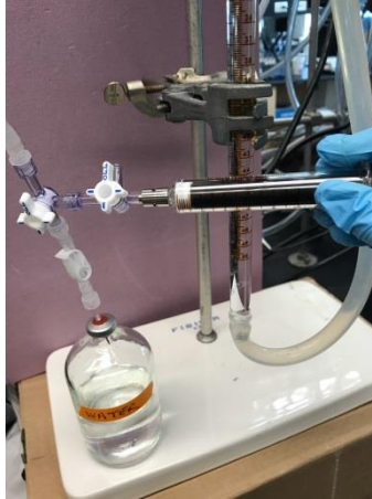
Figure 3.4 Stopcock “off” position when drawing gas sample for composition analysis.
