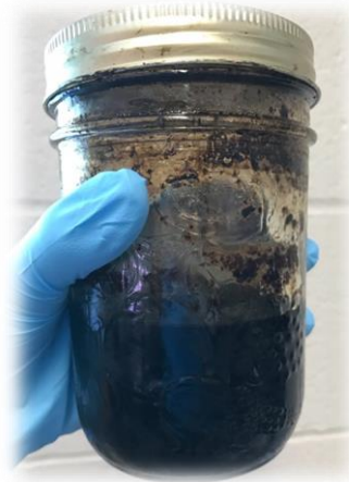
Figure 3.1 Aqueous Pyrolysis Condensate (APC) from pyrolysis of Birch bark sawdust at 500 °C.
