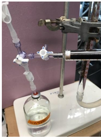
Figure 3.5 Stopcock “off” position when finishes drawing gas sample for composition analysis.
