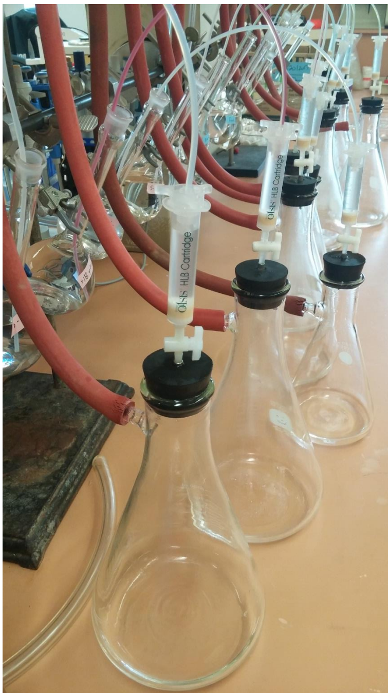
Figure 9: SPE setup for three samples Volumes measured in volumetric flasks on the left and using vacuum pressure to allow a controlled interaction with the stationary phase (1 drop/sec)
