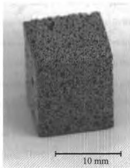
**Figure 2-1: Porous titanium sample.**
