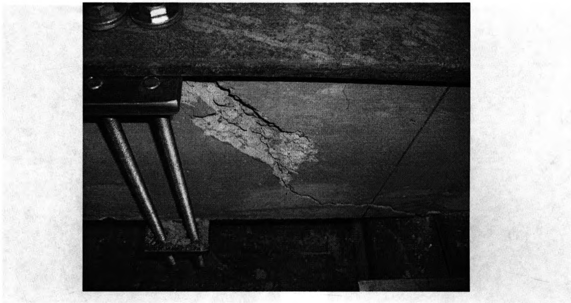
Fig. 3.12: Typical shear failure of the control as-built RC beam specimen.
