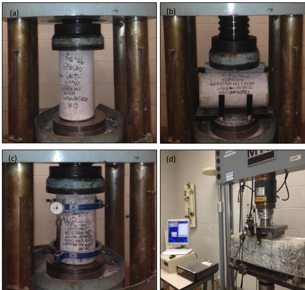
Figure 3.5: Illustration of mechanical testing: (a) compressive strength; (b) splitting tensile strength; (c) modulus of elasticity; and (d) flexural strength.
