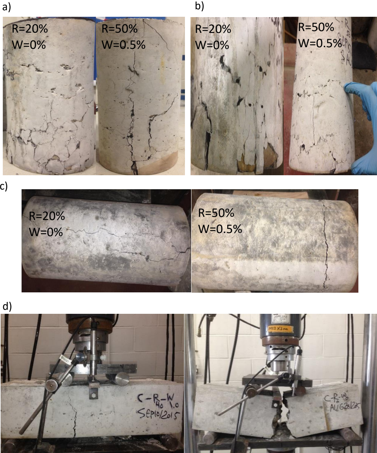
Figure 3.12: Failure mode of specimens with and without waste steel-wires in: (a) compressive testing; (b) modulus of elasticity testing; (c) splitting tensile testing; and (d) flexural testing.
