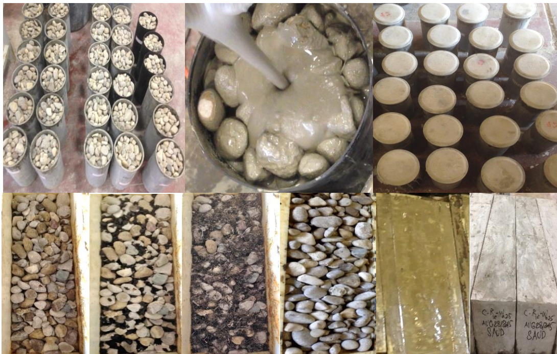
Figure 3.3: Preparation of cylindrical and beam specimens.
