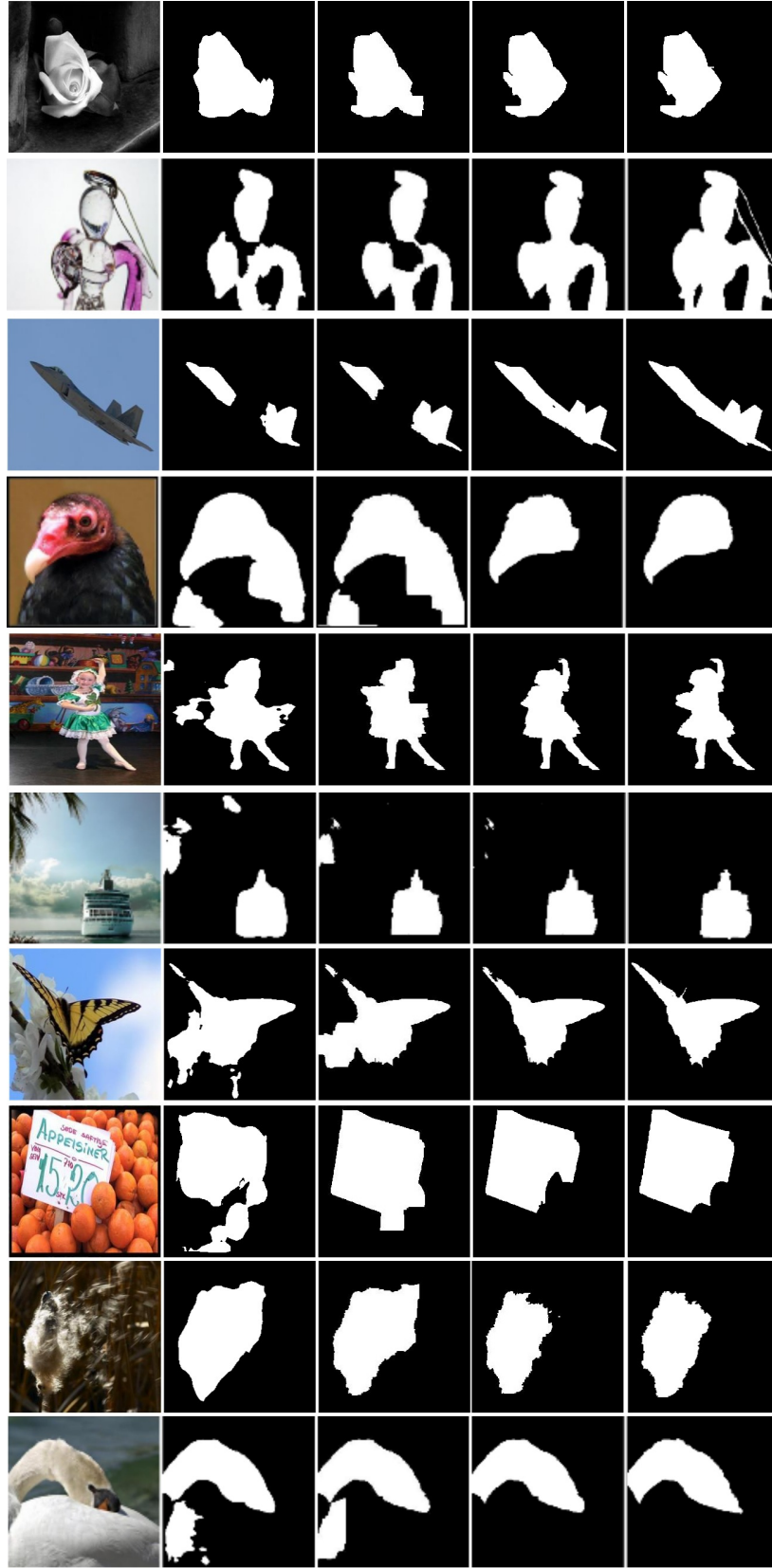
Figure 4.3: Some successful examples. From left to right: original image, segmentation produced by saliency-CNN, segmentation of CNN+CRF with the same regularization weight \lambda_{fixed} for all images, segmentation of CNN+CRF with \lambda_{pred} learned by our weight-CNN, ground truth
