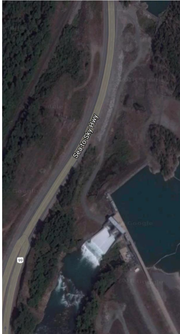
Figure 21: Aerial Photograph of the Cheakamus Dam Emergency Spillway Vegetation (after Google Maps January 2018)
