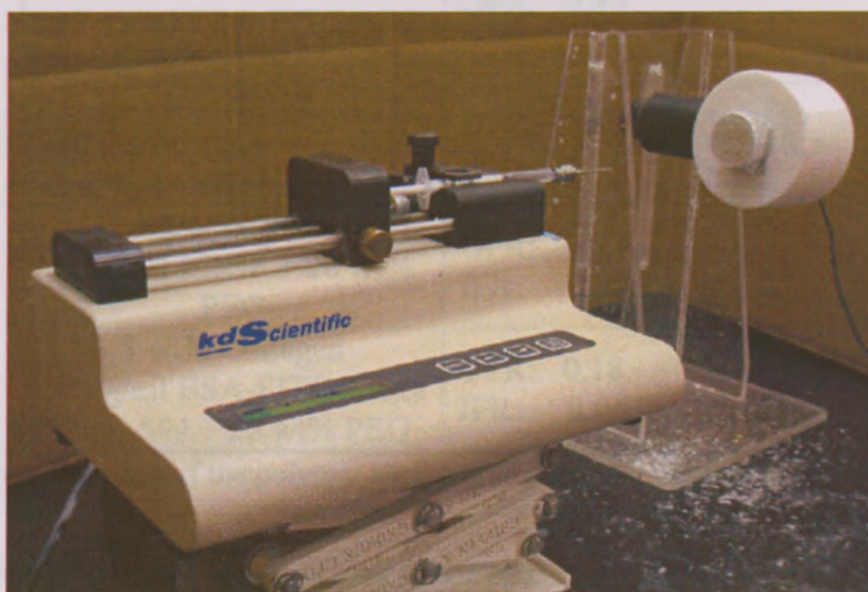
Figure 3.1: Custom designed electrospinning setup.
