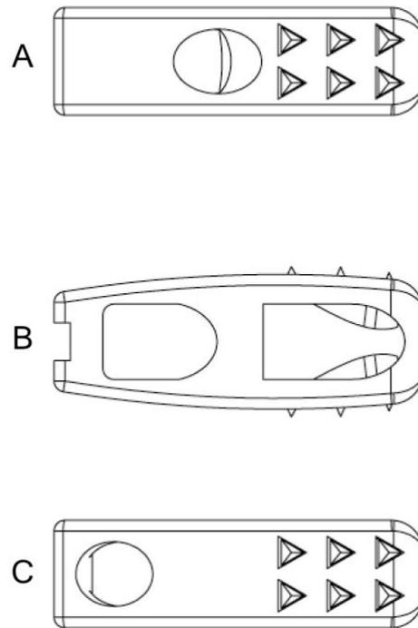
**Figure 1:** Computer assisted drawing of : A) upper view of the stand-alone cage
