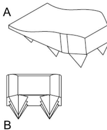
**Figure 2:** Computer assisted drawing of the spike system inside the cage.
