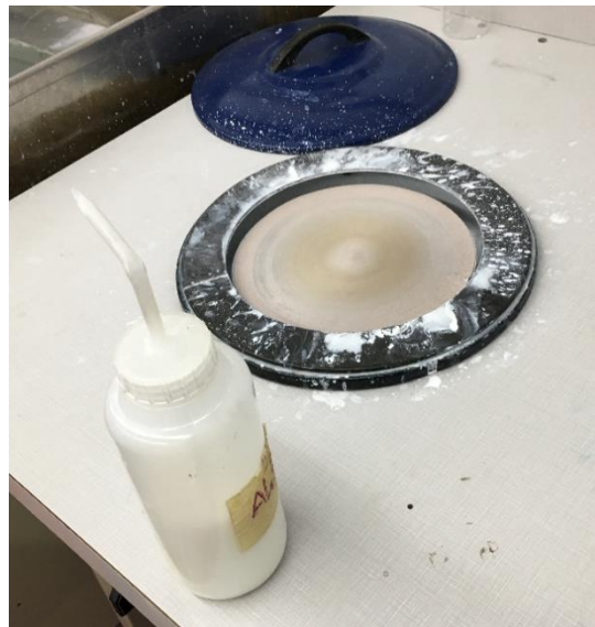
Figure 3.13 polishing machine and polishing powder for the C/DFRC specimen.
