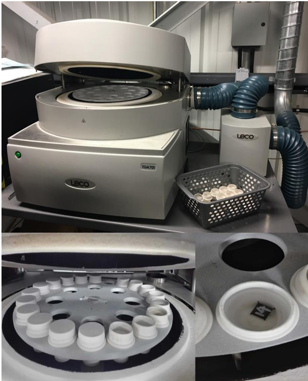
Figure 3.8 Burn-off test equipment.
