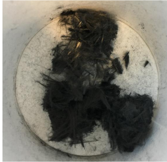
Figure 3.10 The remaining carbon fibers after burn-off test.
