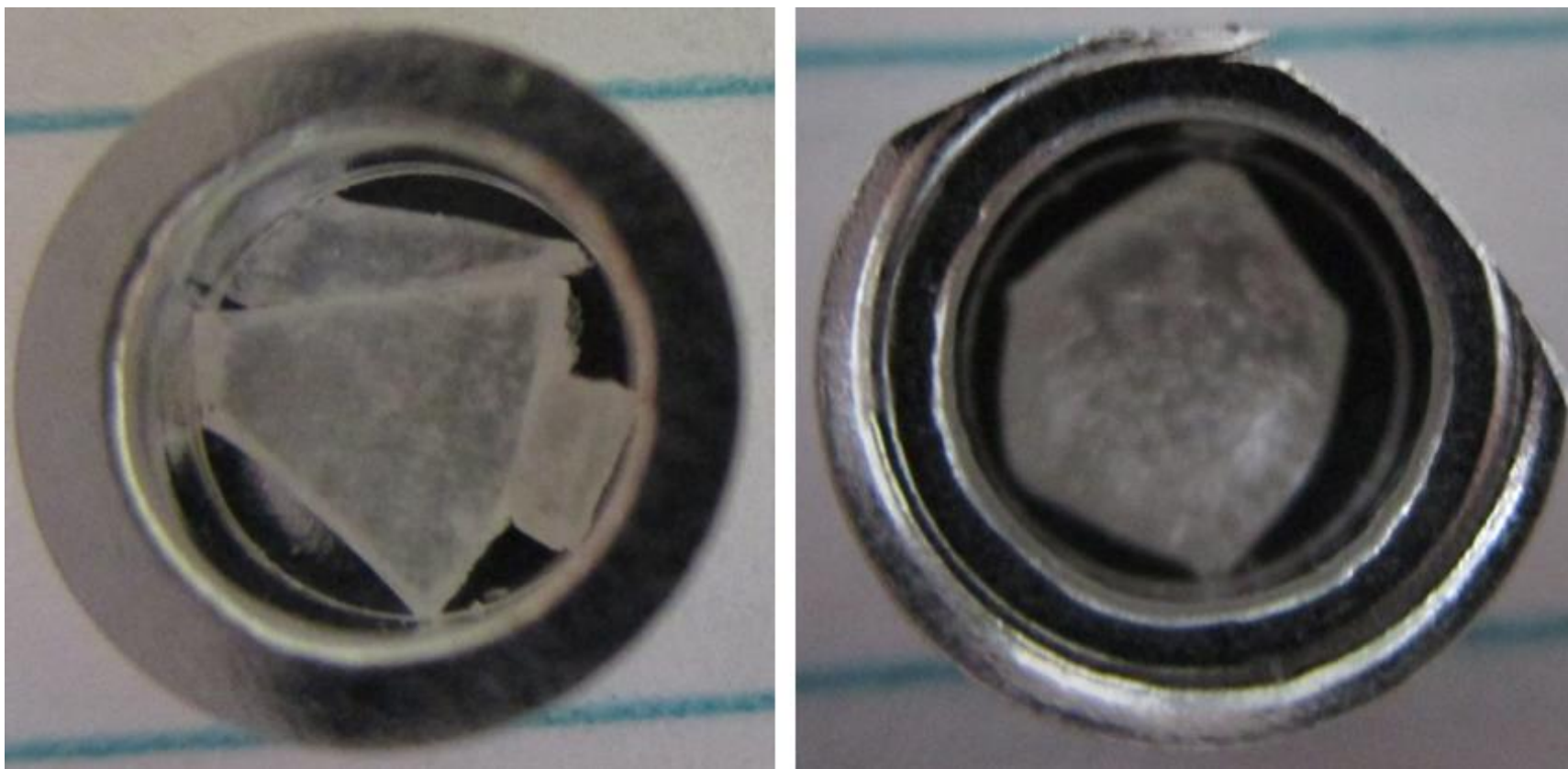
Figure 93. Photographs of Sample 7C, after originally being put into the DSC pan (left) and after testing when the lid was removed (right). This sample has a floor-based shape.
