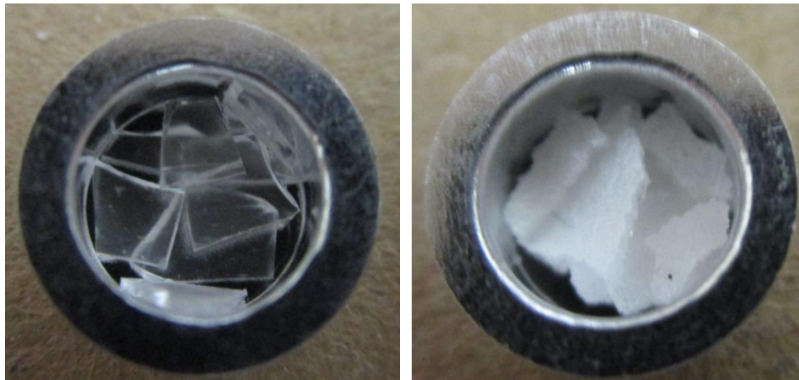
Figure 62. Samples before heating. On the left is a sample of neat PMMA without solvent; on the right is a solvent-containing composite sample.
