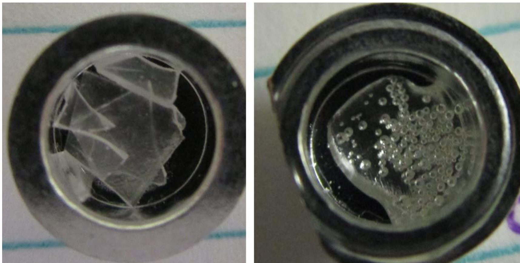
Figure 108. Photographs of Sample 22C, after originally being put into the DSC pan (left) and after testing when the lid was removed (right). This sample has a floor-based shape.
