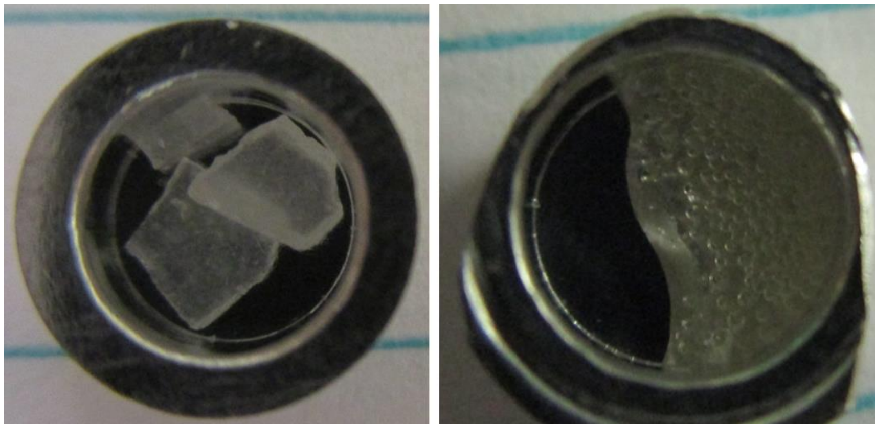
Figure 105. Photographs of Sample 19C, after originally being put into the DSC pan (left) and after testing when the lid was removed (right). This sample exhibits slight yellowing and a floor-based shape.
