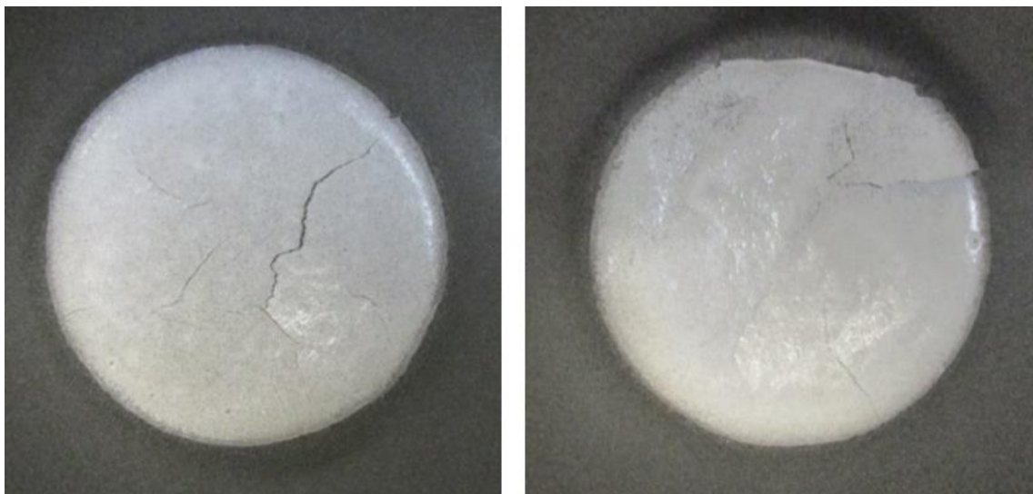
Figure 6. Solvent-containing PMMA (left) and solvent-containing composite (right) samples from Study 3; no images from Study 1 are available but they appeared similar. The composite sample looks very similar to the PMMA sample.
