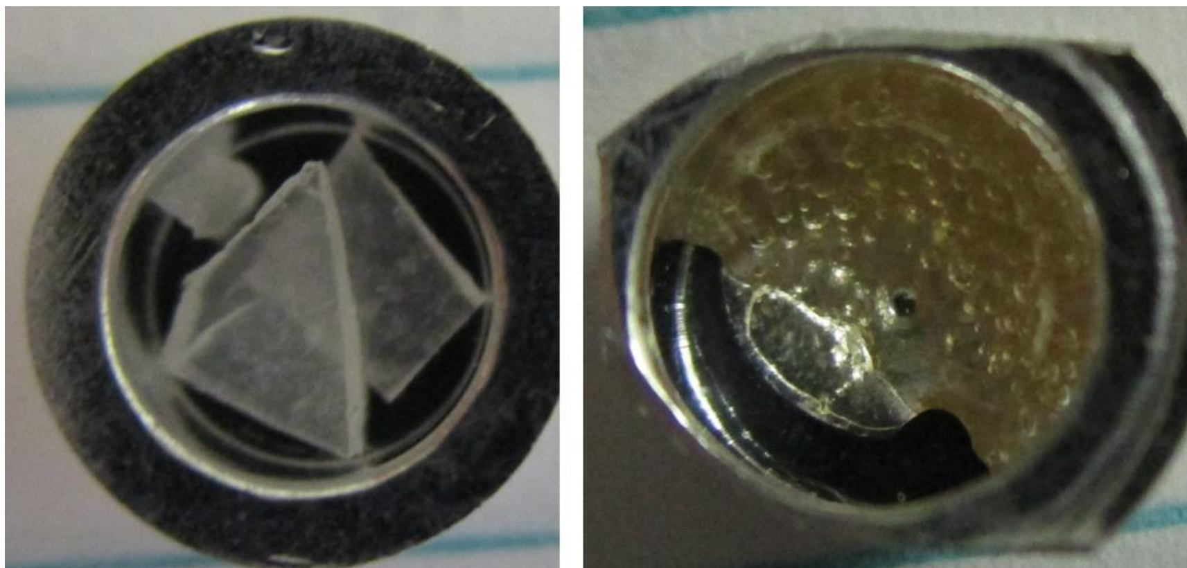
Figure 107. Photographs of Sample 21C, after originally being put into the DSC pan (left) and after testing when the lid was removed (right). This sample exhibits yellowing and a floor-based shape.
