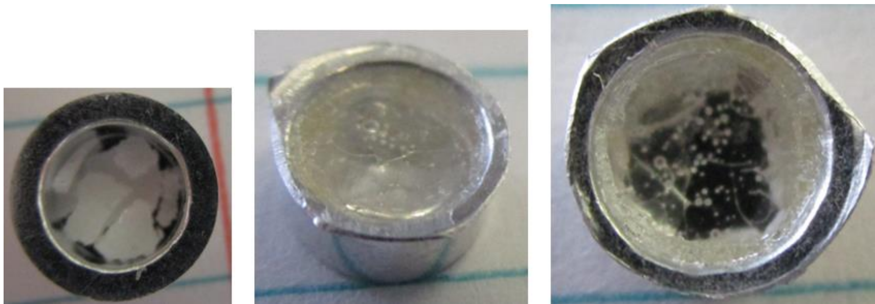
Figure 88. Photographs of Sample 2C, after originally being put into the DSC pan (left), after testing when the lid was removed (center), and after pressing in the roof of the structure to reveal the hollowness inside (right). This sample has a single compartment capsule shape.
