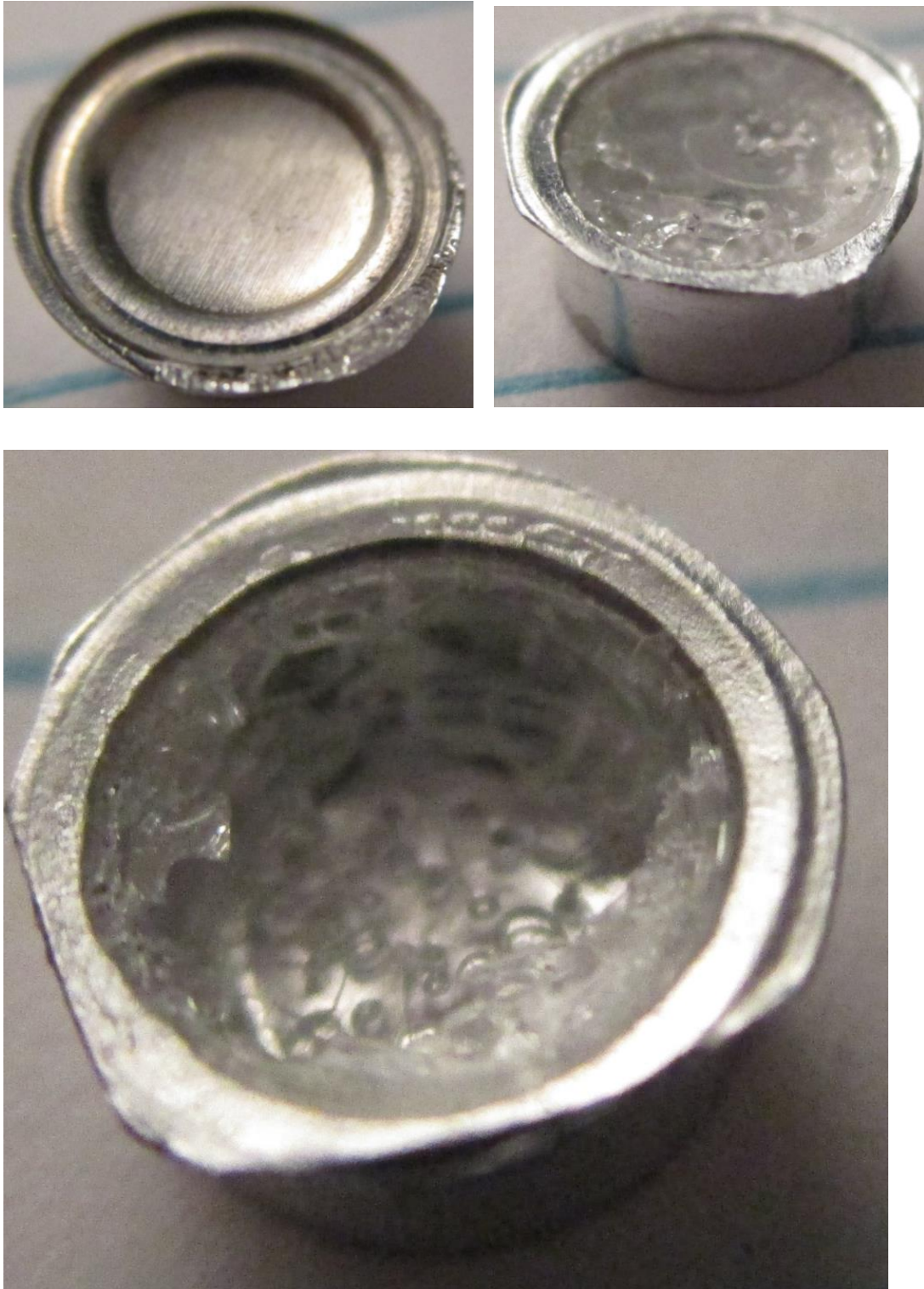
Figure 74. Photographs of Sample 13B, showing pan leakage (top left), intact structure (top right), and structure after pressing in roof to reveal hollow center (bottom). This sample has a capsule shape.
