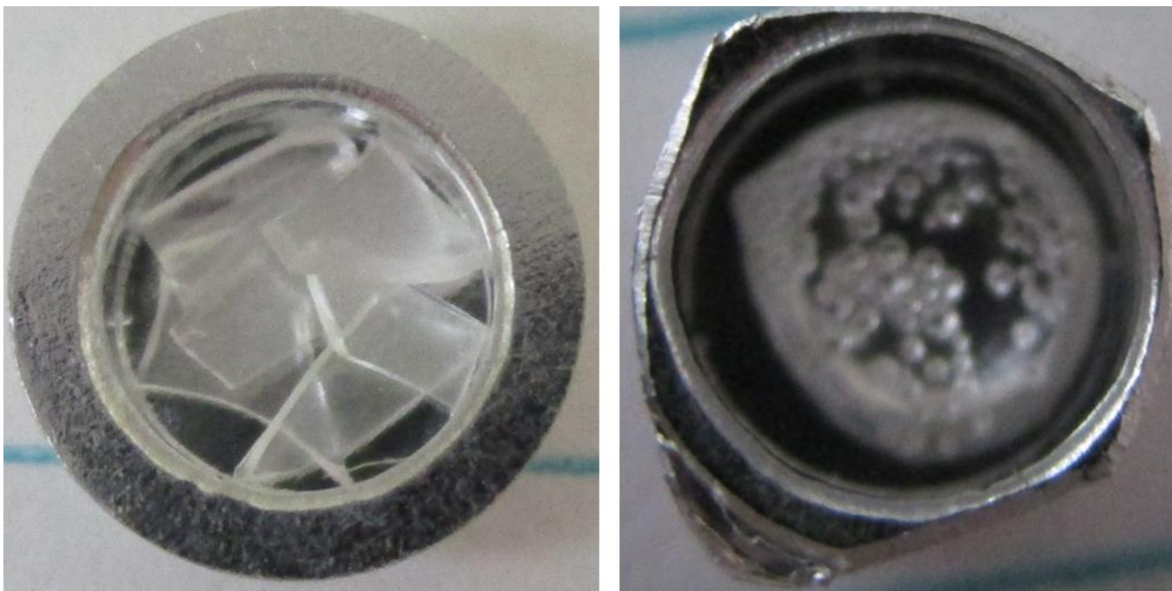
Figure 98. Photographs of Sample 12C, after originally being put into the DSC pan (left) and after testing when the lid was removed (right). This sample has a floor-based shape.
