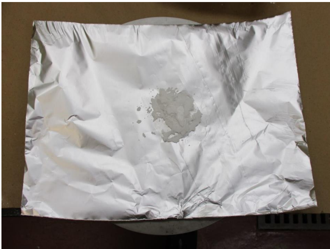
Figure 1. Powder on aluminum foil, on a metal disc, that would later be covered with another piece of aluminum foil before being transferred to the melt press.
