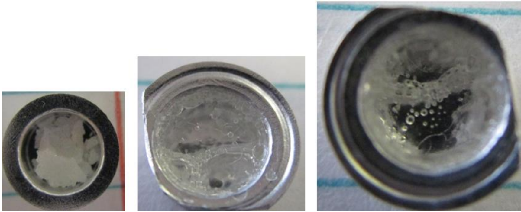
Figure 90. Photographs of Sample 4C, after originally being put into the DSC pan (left), after testing when the lid was removed (center), and after pressing in the roof of the structure to reveal the hollowness inside (right). This sample has a multi-compartment capsule shape.
