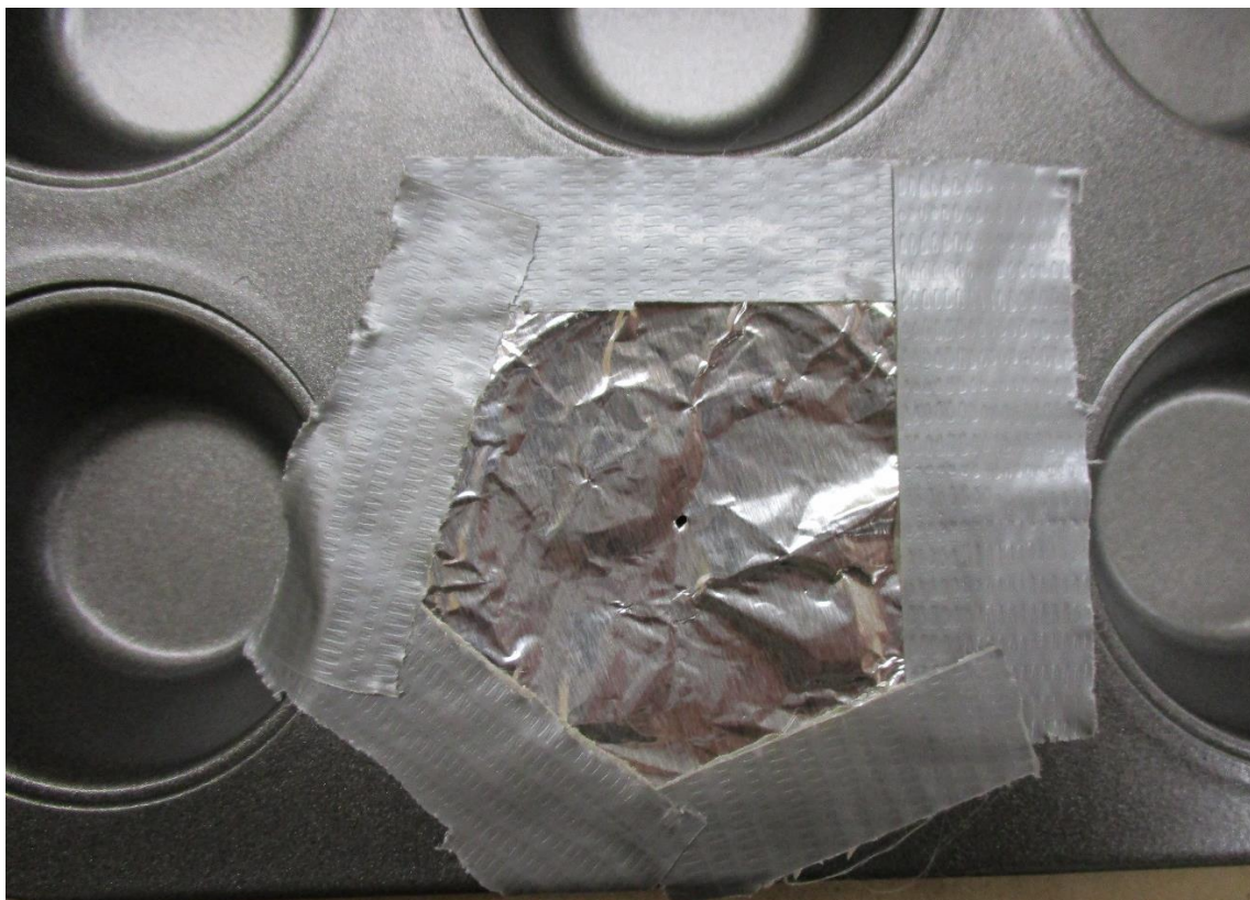
Figure 3. Example of a baking tray compartment sealed with aluminum foil and duct tape. The compartment contains a sample of PMMA or composite together with acetone. A small hole is present in the middle of this makeshift lid to allow for acetone evaporation.
