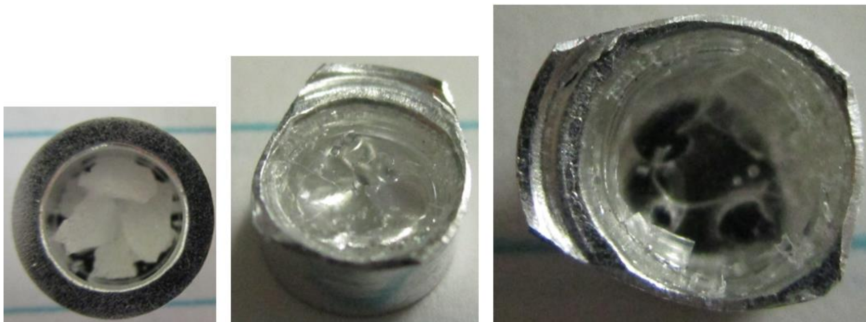
Figure 102. Photographs of Sample 16C, after originally being put into the DSC pan (left), after testing when the lid was removed (center), and after pressing in the roof of the structure to reveal the hollowness inside (right). This sample has a single compartment capsule shape.
