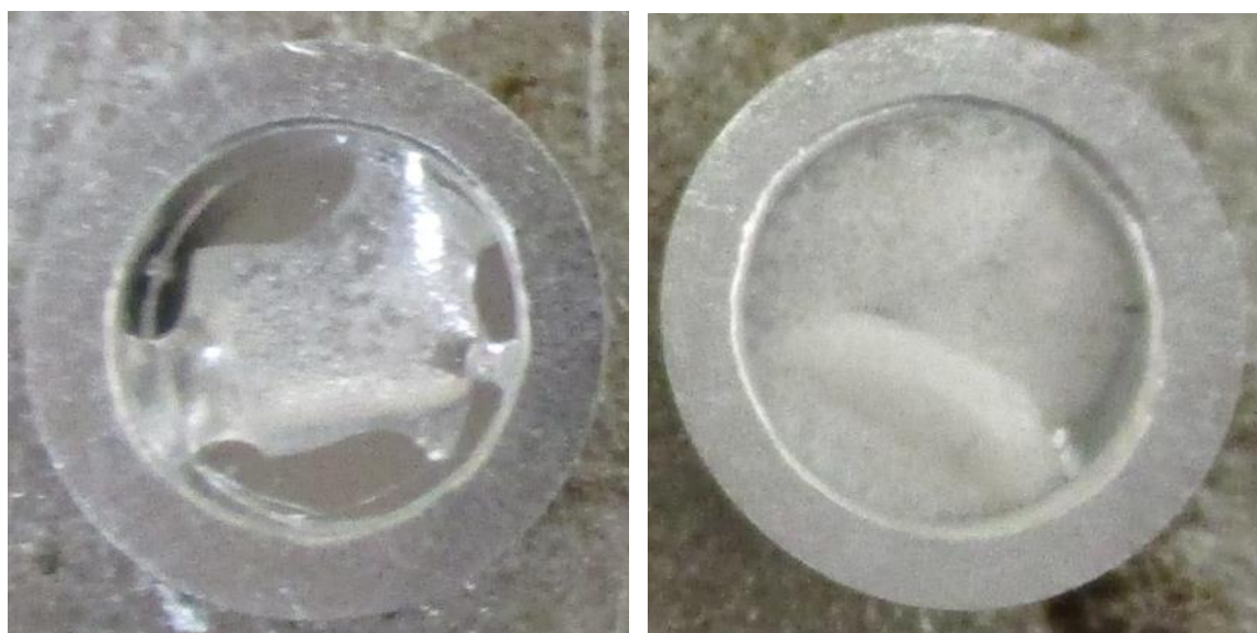
Figure 63. Samples at the same time partway through heating. On the left is neat PMMA without solvent; on the right is the solvent-containing composite. The latter is seen to have expanded.
