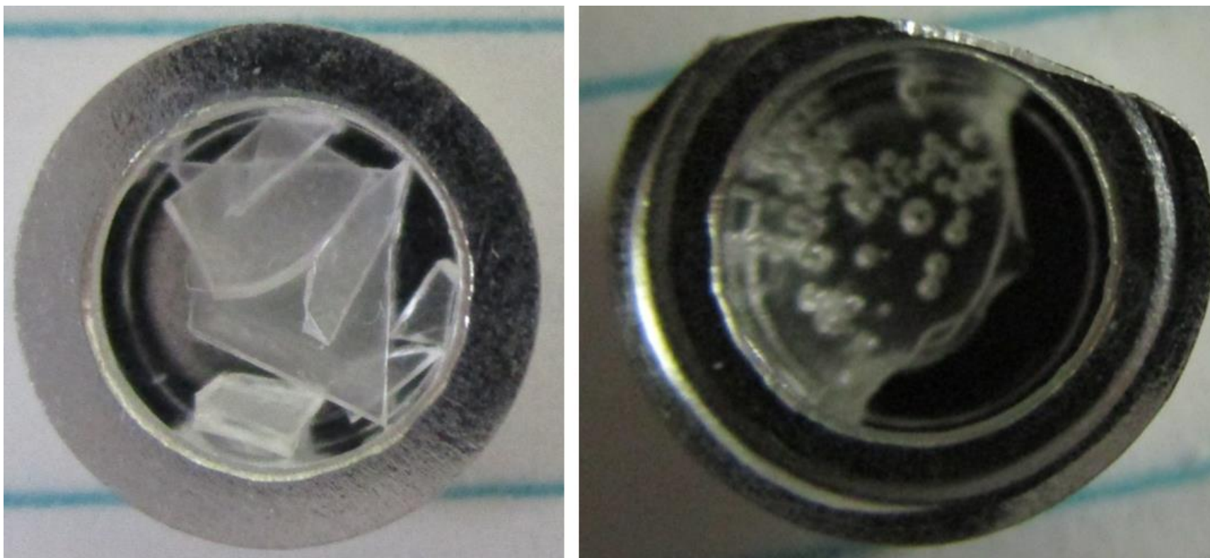
Figure 109. Photographs of Sample 23C, after originally being put into the DSC pan (left) and after testing when the lid was removed (right). This sample has a floor-based shape.
