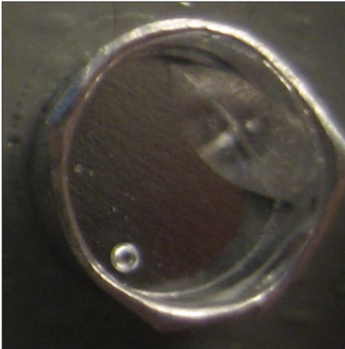
Figure 18. Top view of opened DSC pan of the outlier sample (P160 condition; Sample ID #11 in Appendix A). The sample is convex, with minimal contact with the pan floor.
