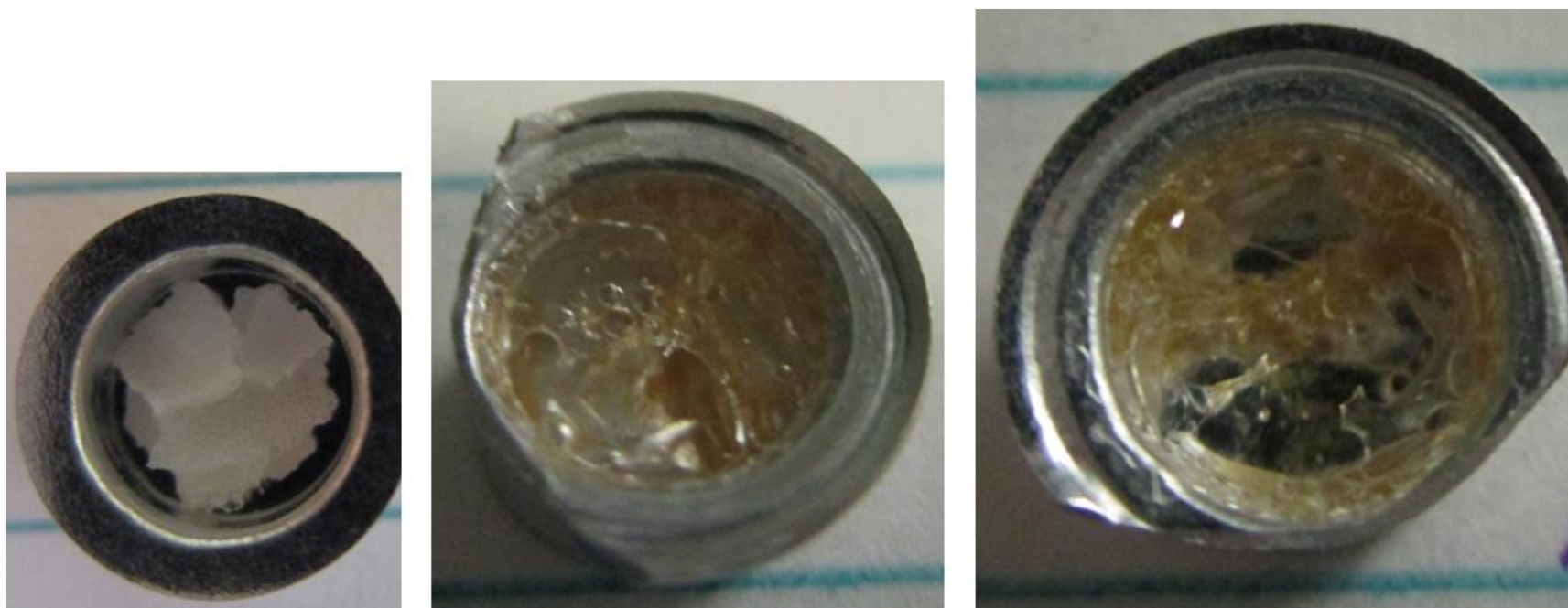
Figure 101. Photographs of Sample 15C, after originally being put into the DSC pan (left), after testing when the lid was removed (center), and after pressing in the roof of the structure to reveal the hollowness inside (right). This sample exhibits yellowing and a multi-compartment capsule shape.
