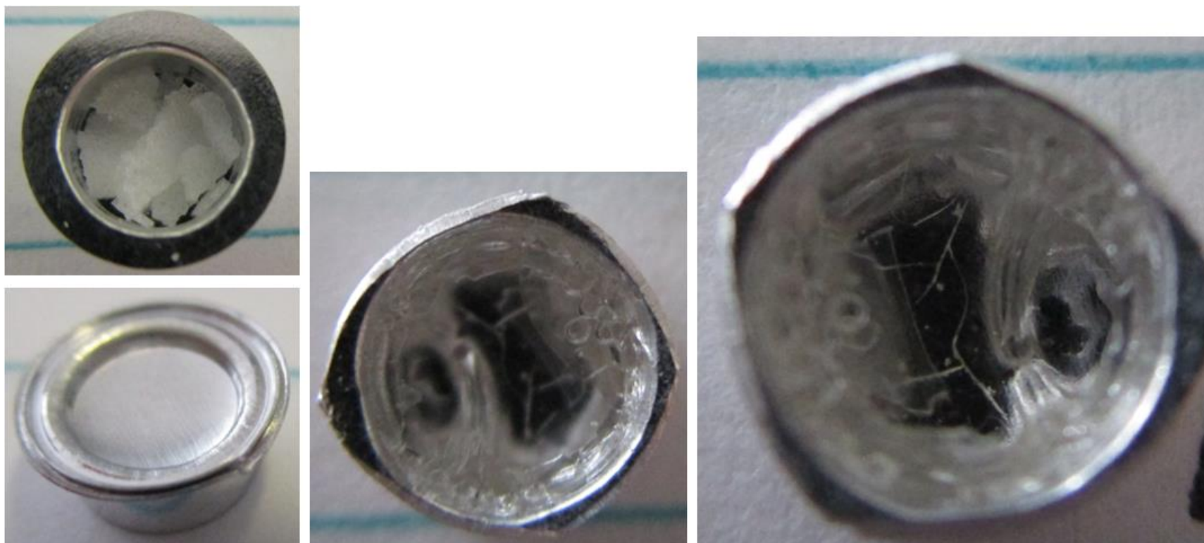
Figure 99. Photographs of Sample 13C, after originally being put into the DSC pan (left top), after testing before the lid was removed – a dent is seen (left bottom), after the lid was removed (center), and after pressing in the roof of the structure to reveal the hollowness inside (right). This sample has a multi-compartment capsule shape.
