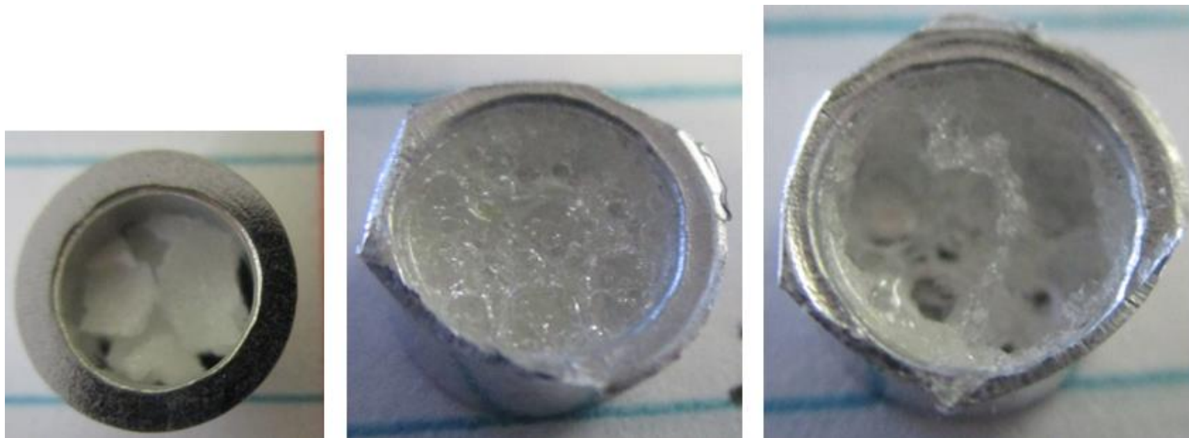
Figure 87. Photographs of Sample 1C, after originally being put into the DSC pan (left), after testing when the lid was removed (center), and after pressing in the roof of the structure to reveal the hollowness inside (right). This sample has a multi-compartment capsule shape.
