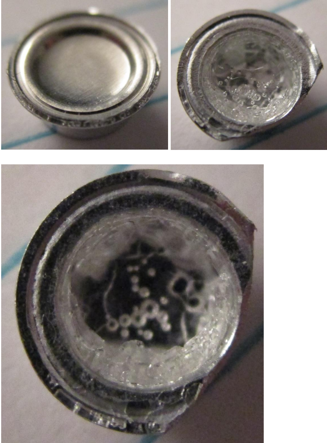
Figure 82. Photographs of Sample 21B, showing pan leakage (top left), intact structure (top right), and structure after pressing in roof to reveal hollow center (bottom). This sample has a capsule shape.
