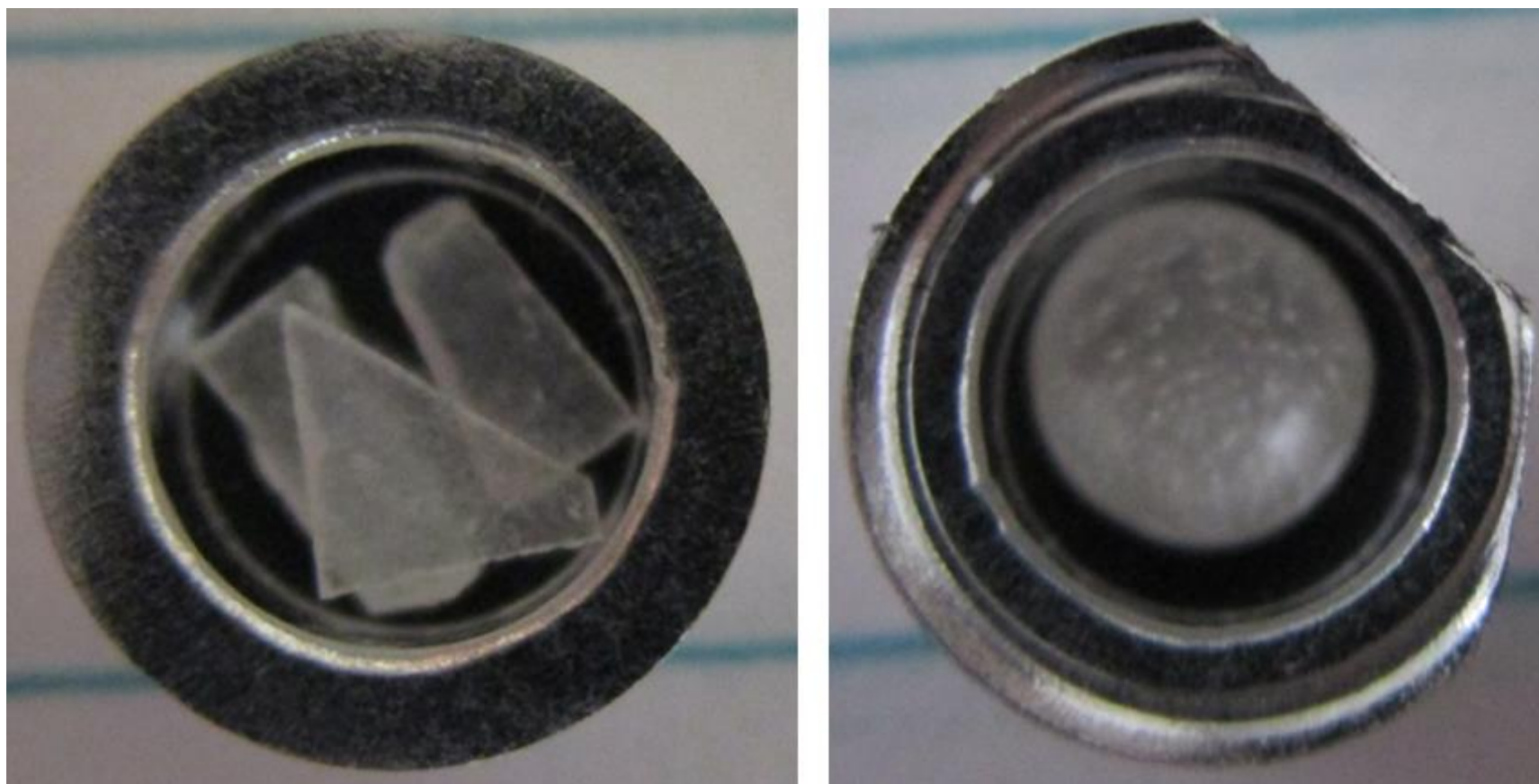
Figure 94. Photographs of Sample 8C, after originally being put into the DSC pan (left) and after testing when the lid was removed (right). This sample has a floor-based shape.
