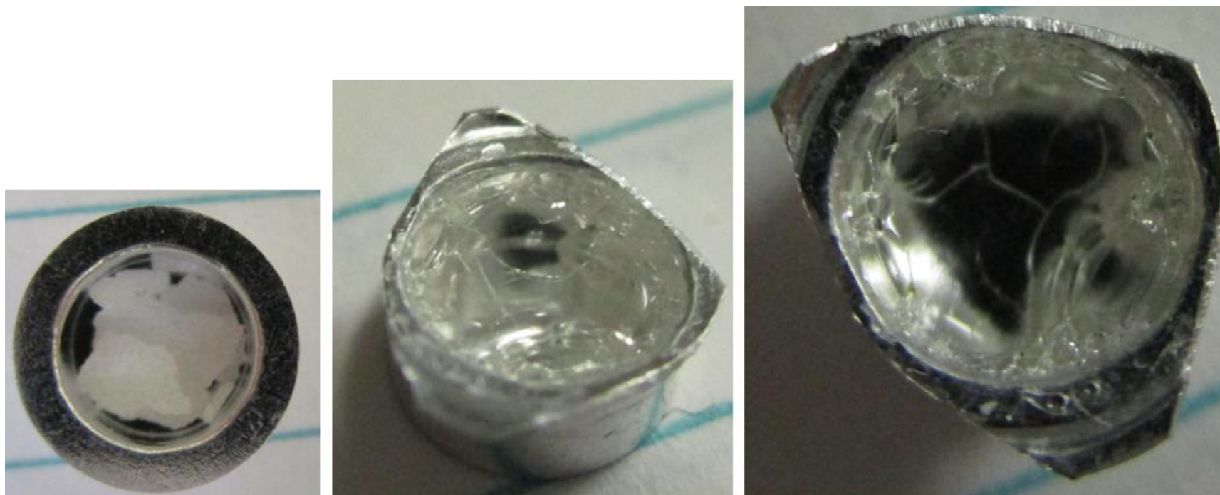
Figure 103. Photographs of Sample 17C, after originally being put into the DSC pan (left), after testing when the lid was removed (center), and after pressing in the roof of the structure to reveal the hollowness inside (right). This sample has a multi-compartment capsule shape.
