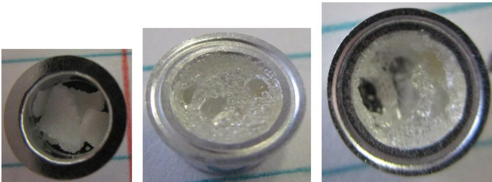
Figure 89. Photographs of Sample 3C, after originally being put into the DSC pan (left), after testing when the lid was removed (center), and after pressing in the roof of the structure to reveal the hollowness inside (right). This sample has a multi-compartment capsule shape.
