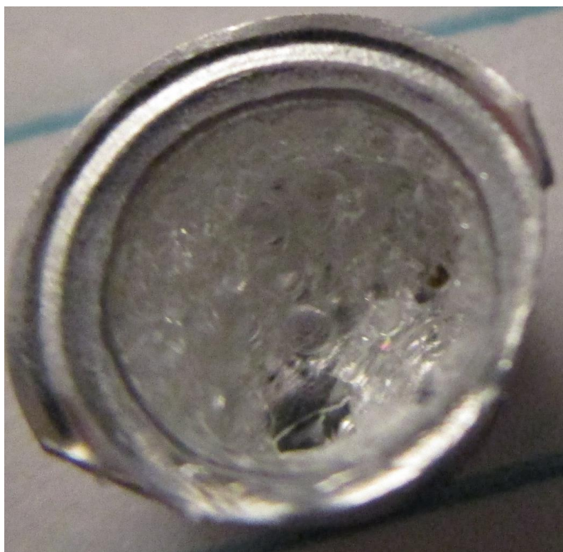
Figure 75. Photographs of Sample 14B, showing intact structure (top) and structure after pressing in roof to reveal hollow center (bottom). This sample has a capsule shape.
