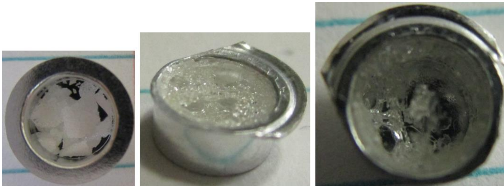
Figure 104. Photographs of Sample 18C, after originally being put into the DSC pan (left), after testing when the lid was removed (center), and after pressing in the roof of the structure to reveal the hollowness inside (right). This sample has a multi-compartment capsule shape.
