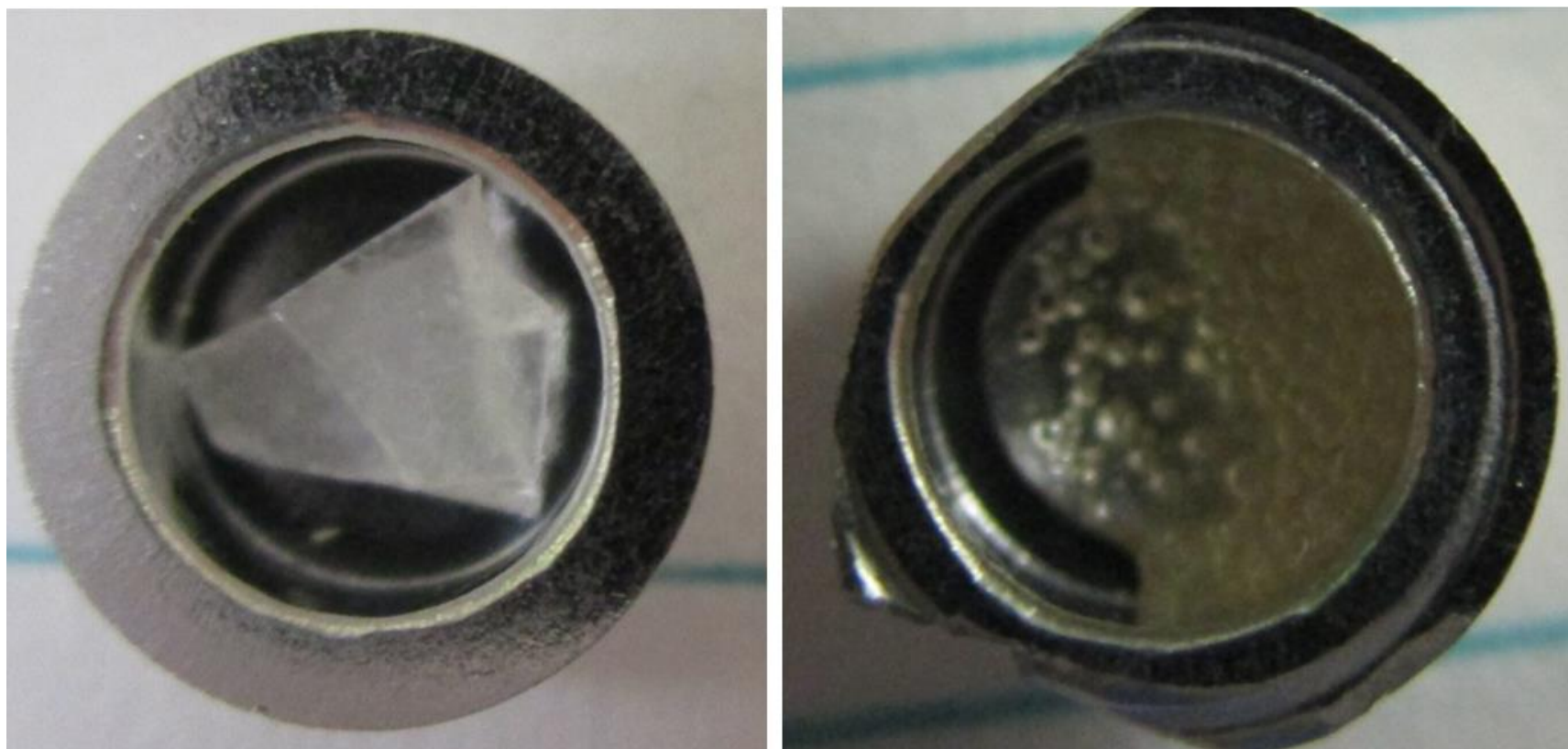
Figure 106. Photographs of Sample 20C, after originally being put into the DSC pan (left) and after testing when the lid was removed (right). This sample exhibits slight yellowing and a floor-based shape.
