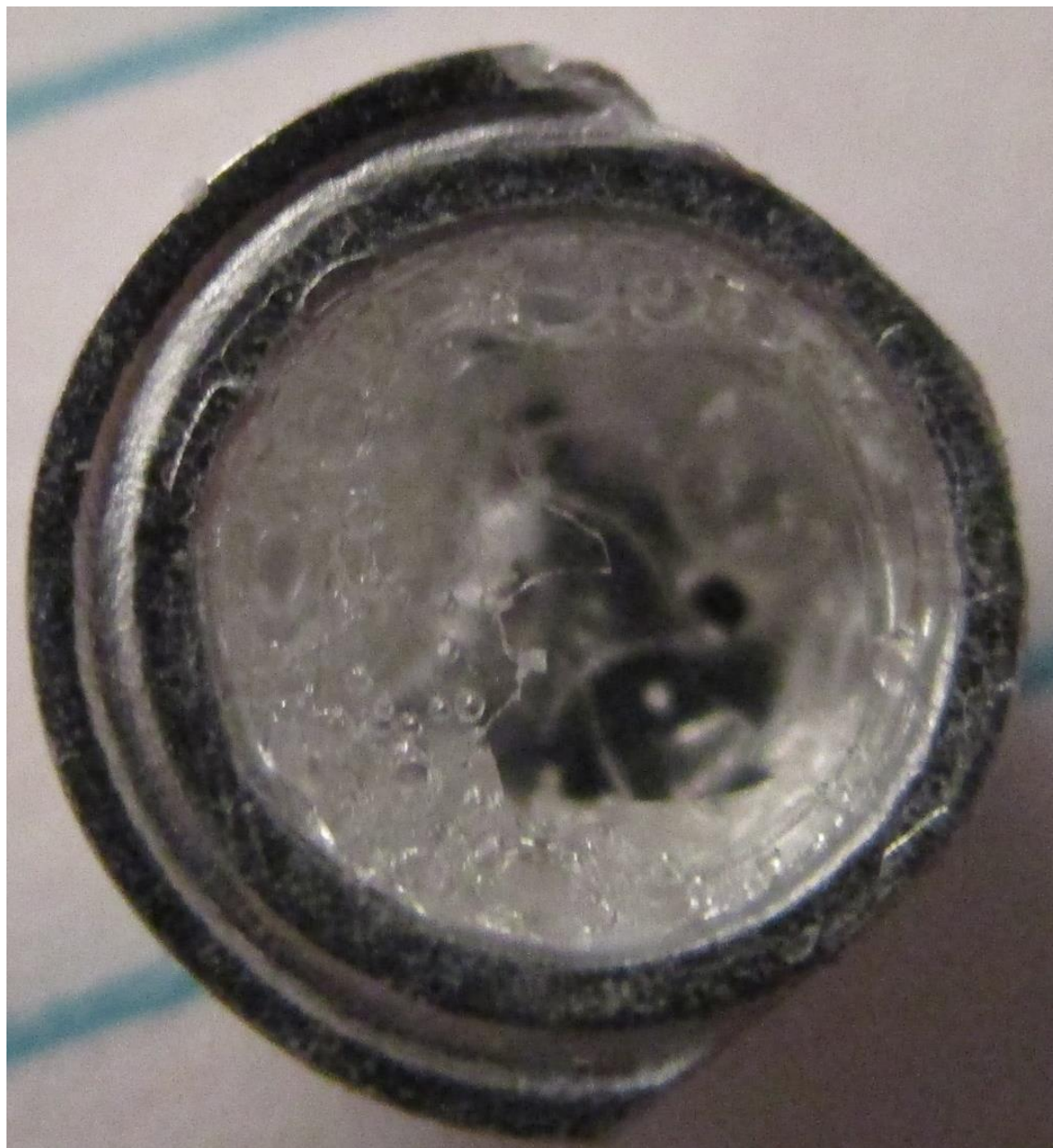
Figure 72. Photograph of Sample 11B, with its roof pushed in to reveal a hollow center. This sample has a capsule shape.
