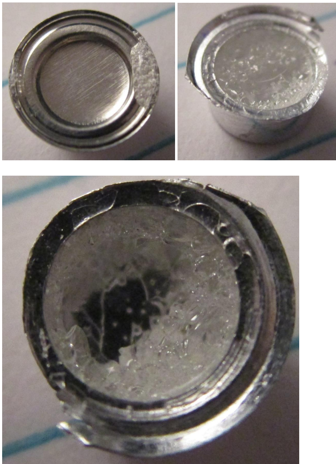
Figure 85. Photographs of Sample 24B, showing pan leakage (top left), intact structure (top right), and structure after pressing in roof to reveal hollow center (bottom). This sample appears to have both a “capsule” and “vertical half” shape.
