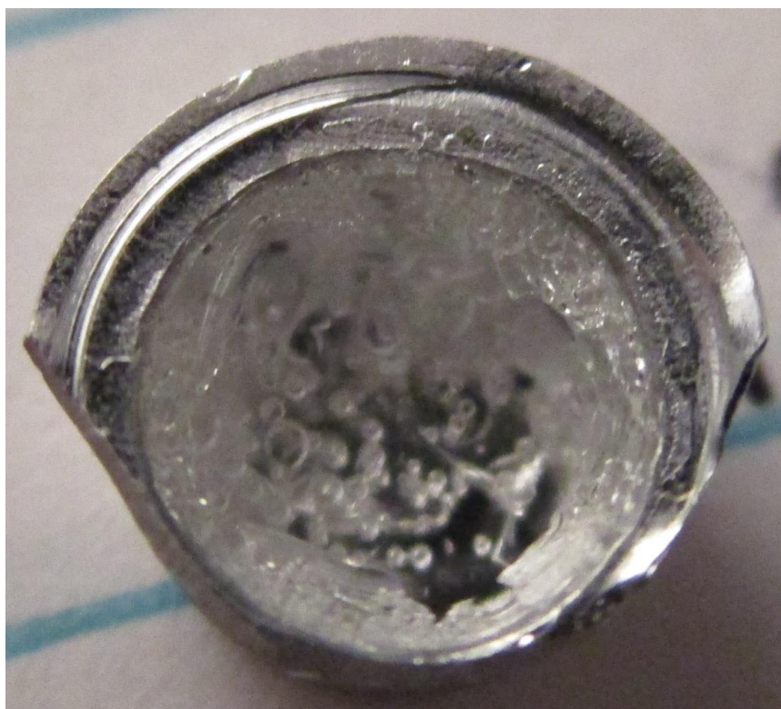
Figure 73. Photographs of Sample 12B, showing intact structure (top) and structure after pressing in roof to reveal hollow center (bottom). This sample has a capsule shape.
