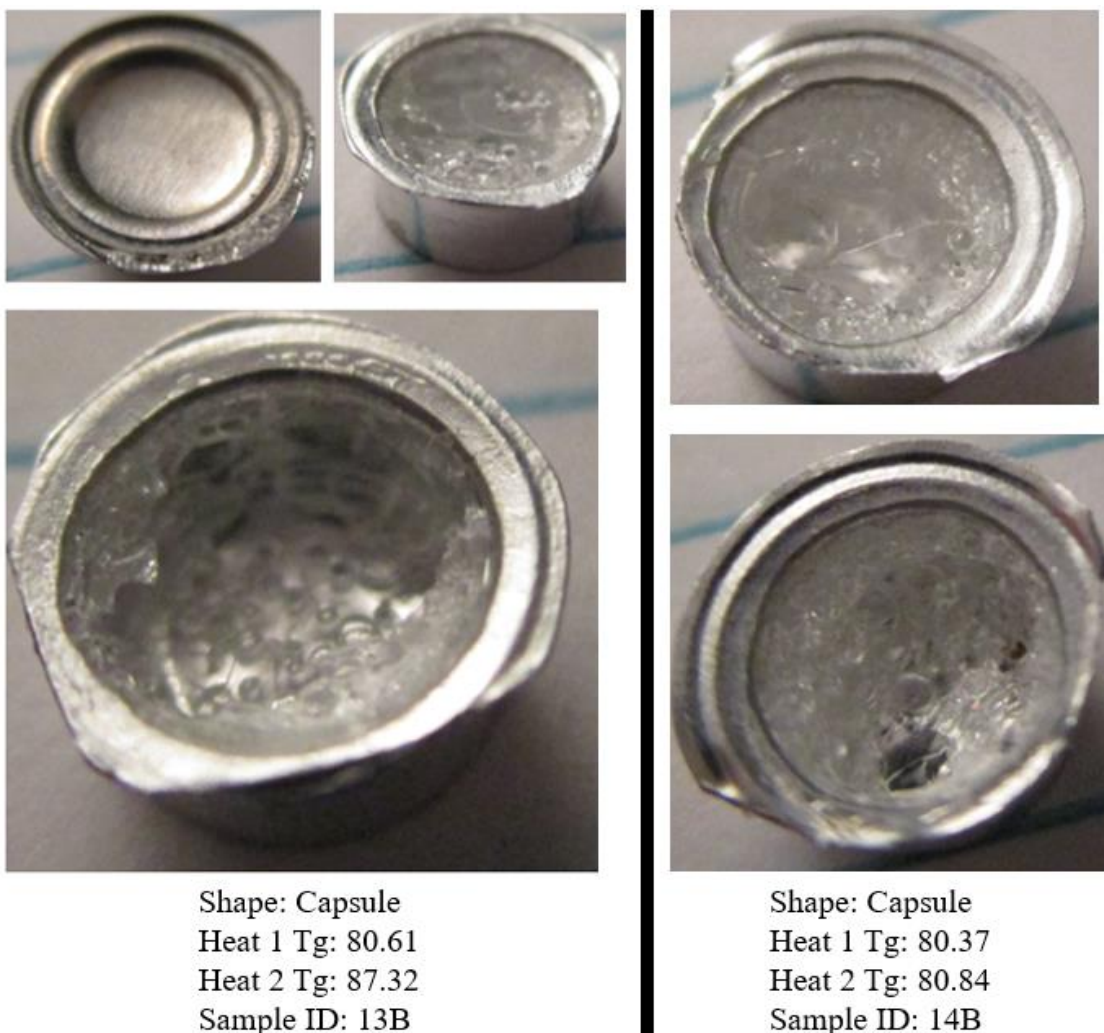
Figure 46. Samples 13B (left of vertical line) and 14B (right of vertical line), which comprise the 15-minute ground, solvent-containing, 10 mg condition. For sample
