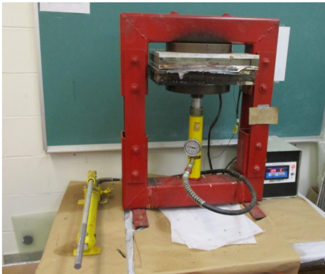
Figure 2. Melt-pressing set-up. The sample powder being pressed is located between two pieces of aluminum foil.
