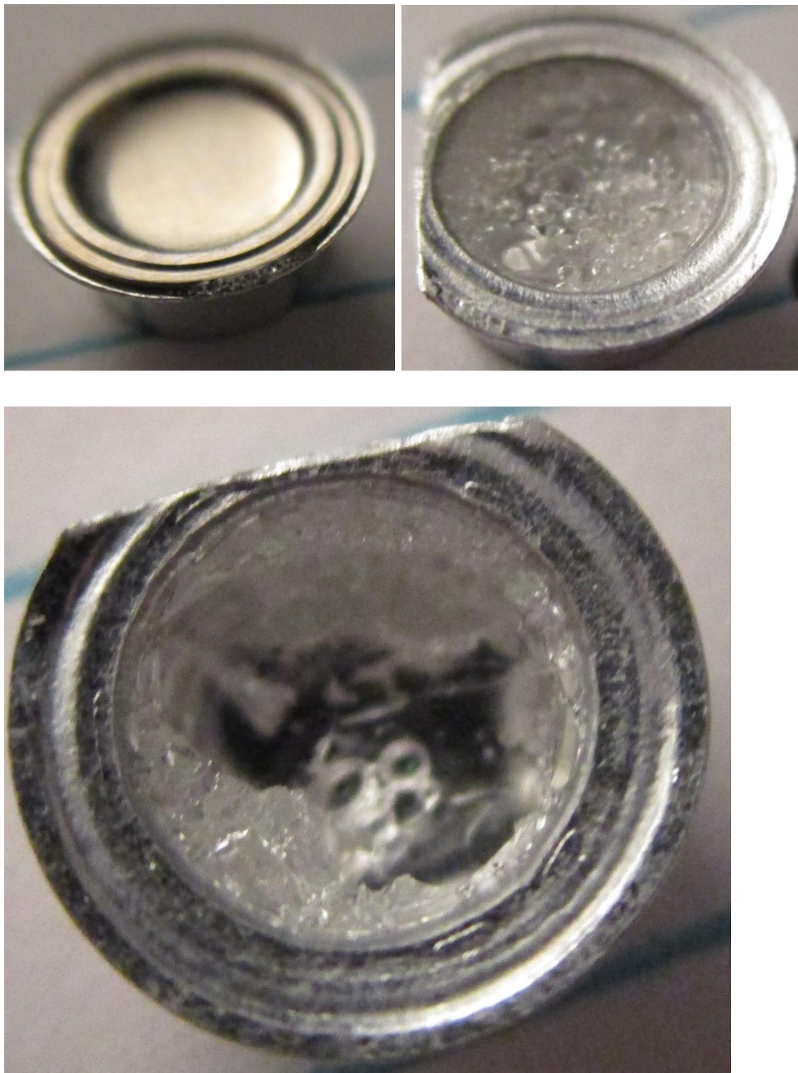
Figure 83. Photographs of Sample 22B, showing pan leakage (top left), intact structure (top right), and structure after pressing in roof to reveal hollow center (bottom). This sample has a capsule shape.
