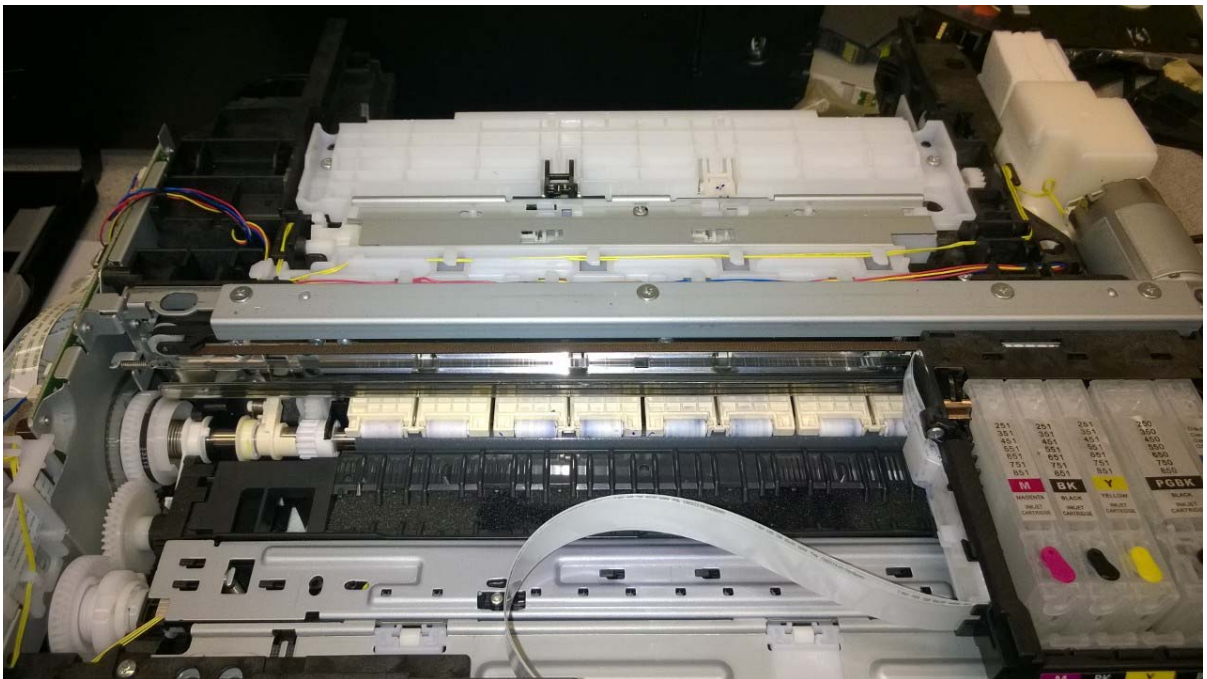
Figure 4.1 Paper feed mechanism of a Canon IP7220 inkjet printer. Office inkjet printers feature rollers to feed paper through and keep it in place during printing process. Regardless of feeding route, paper goes through rollers after inkjet printing.
