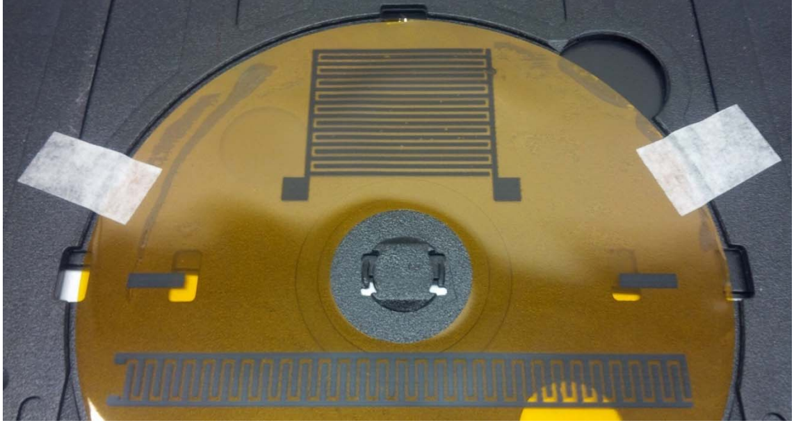
Figure 4.2 Epson 2800 CD/DVD tray. CD/DVD trays allow use of both rigid and flexible substrates. Substrates must be fixed on the surface to avoid shifting during printing and keep flexible substrates from coming into contact with printhead.
