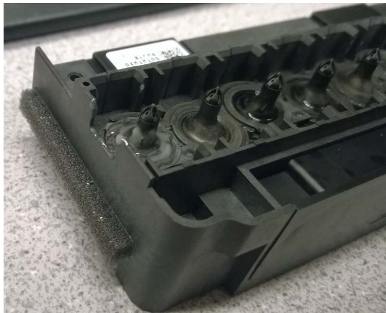
Figure 4.3 Epson R2800 Printhead. Under the conical manifolds, there are thick cellulose filters to prevent contaminants from entering printhead assembly. To be able to use this printhead for inkjet print colloidal inks, cellulose filters must be removed.
