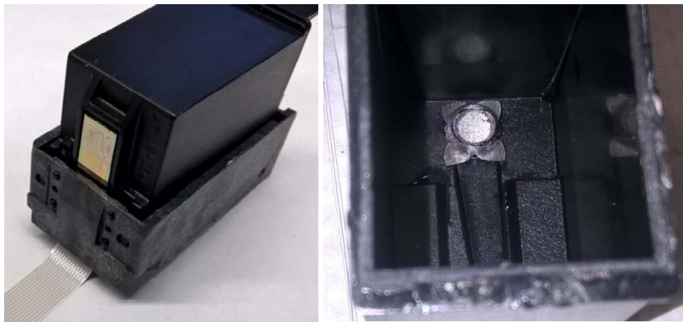
Figure 4.5 HP C6602 Printhead unit and carriage assembly (left). Inside of HP C6602 printhead (right). During this research, metal mesh filter was not removed as G-CMC sheets were small enough to pass through the filter without causing clogging.
