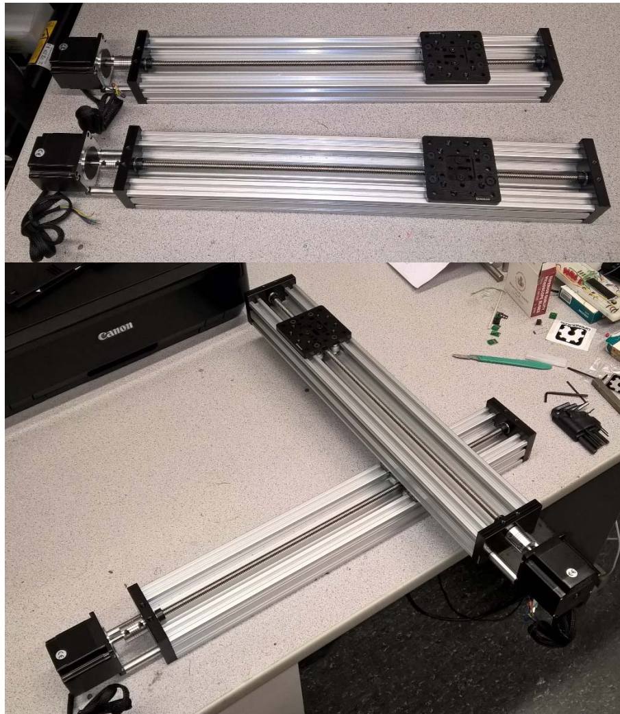
Figure 4.4 C-Beam linear stages with NEMA 23 stepper motors (top). Linear stages can be fixed in 90-degree angle to each other to form an XY coordinate stage (bottom).
