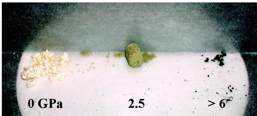
**Figure 1.3: Powdered samples of diiodobutadiyne in an oxalamide host, before pressing (left), after pressing to 2.5 GPa (center), and after pressing to 6 GPa (right). (ref. 8) (Reproduced with the permission of American Chemical Society)**
