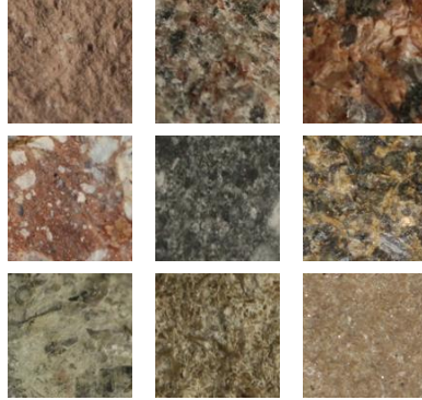
Figure 3.1: Sample images from dataset. Each sample stands for one class. All images have size of 128 \times 128 \times 3 pixels and are between 1 and 2 cm across . From top to bottom, the first column – rhyolite, volcanic breccia, limestone; the second column – granite, andesite, oolitic limestone; the third column – red granite, peridotite, dolostone.
