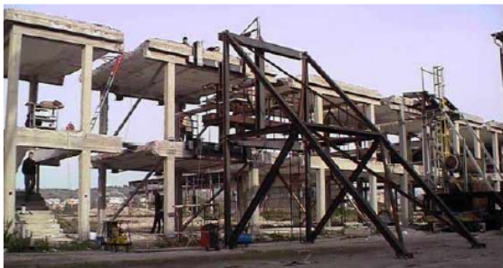
Fig. 2-14: Retrofitting of a two storey RC frame using SMAs (Dolce et al. 2004)
