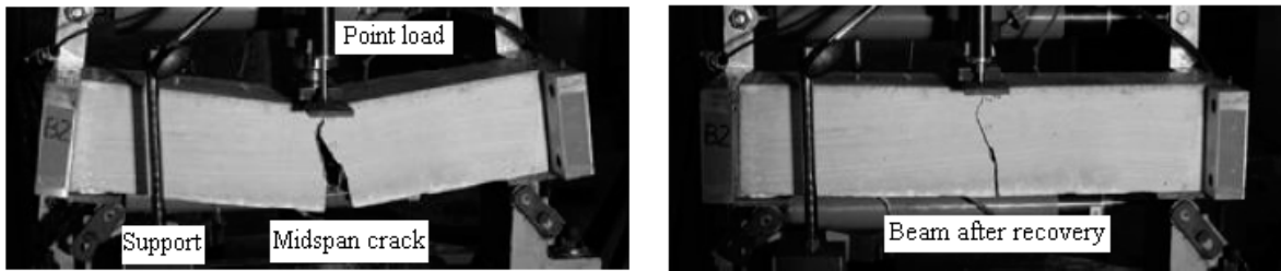
(a) Cracks at maximum deflection
