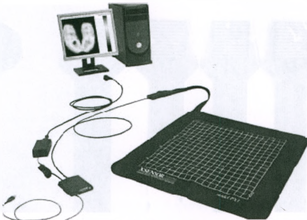
Figure 11 XSensor system including pressure sensing mat, analog to digital converter, power supply, and PC. Adapted from XSensor Technology, 2011.
