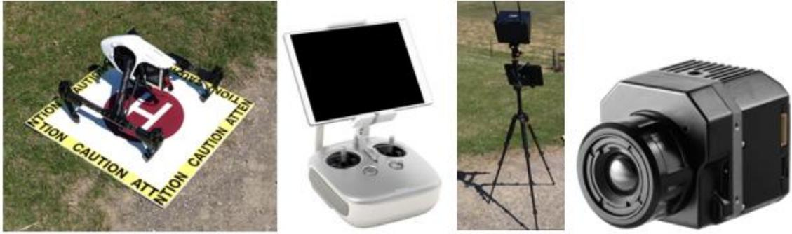
**Figure 7-3: Illustration of the UAV-borne thermal system utilized to scan two RC bridge decks.**
