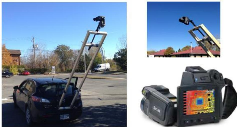
**Figure 4-6: Illustration of the FLIR T650sc IR camera and vehicle mounted setup system utilized to survey Montreal bridge.**
