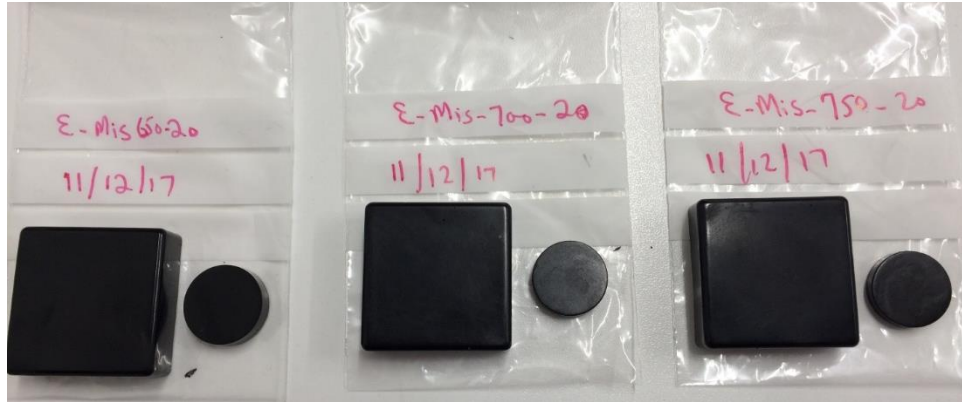
Figure 4.3- Composite for electrical characterization (square) and for other characterizations (cylindrical)
