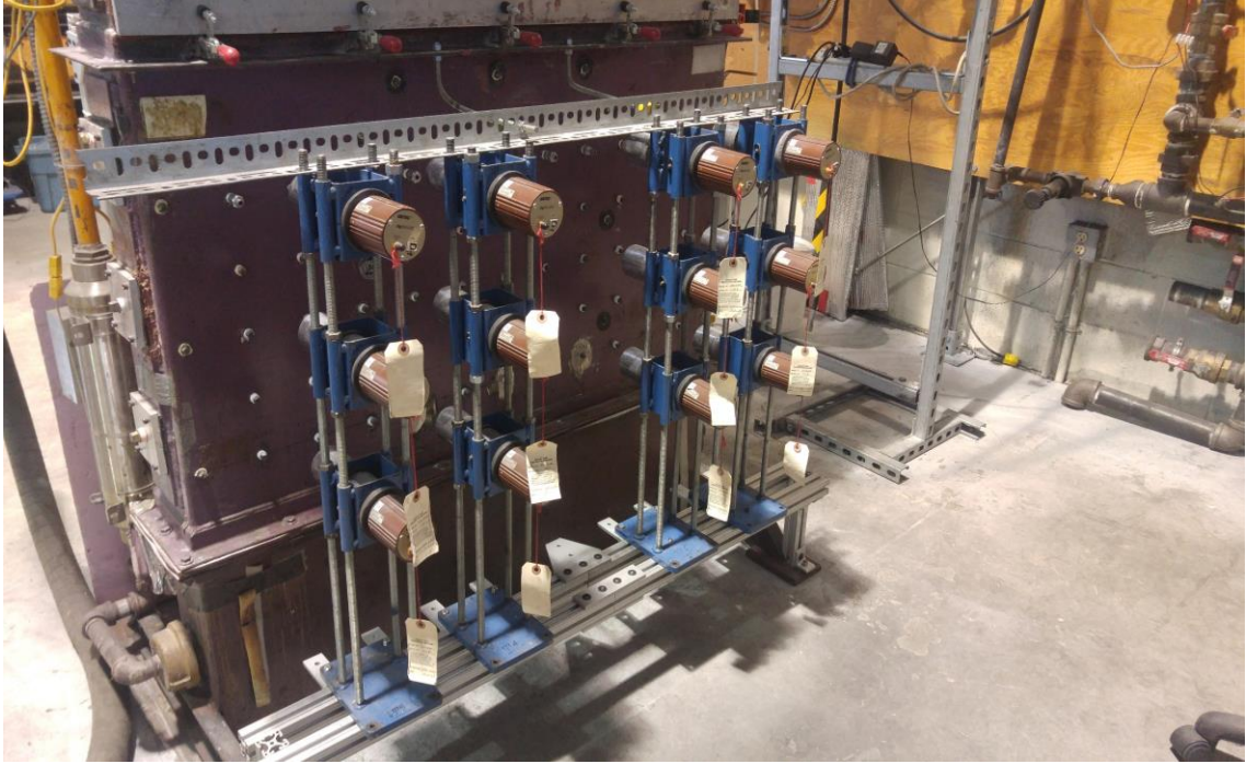
Figure 2-12: Scintillation detectors arranged in 3 x 4 matrix in a 2D plane
