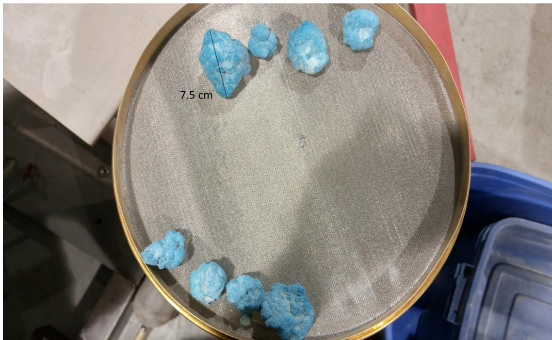
Figure 3-3: Agglomerates larger than 12500 \mu\text{m} collected from the bottom layer at 0.06 m/s fluidization gas velocity
