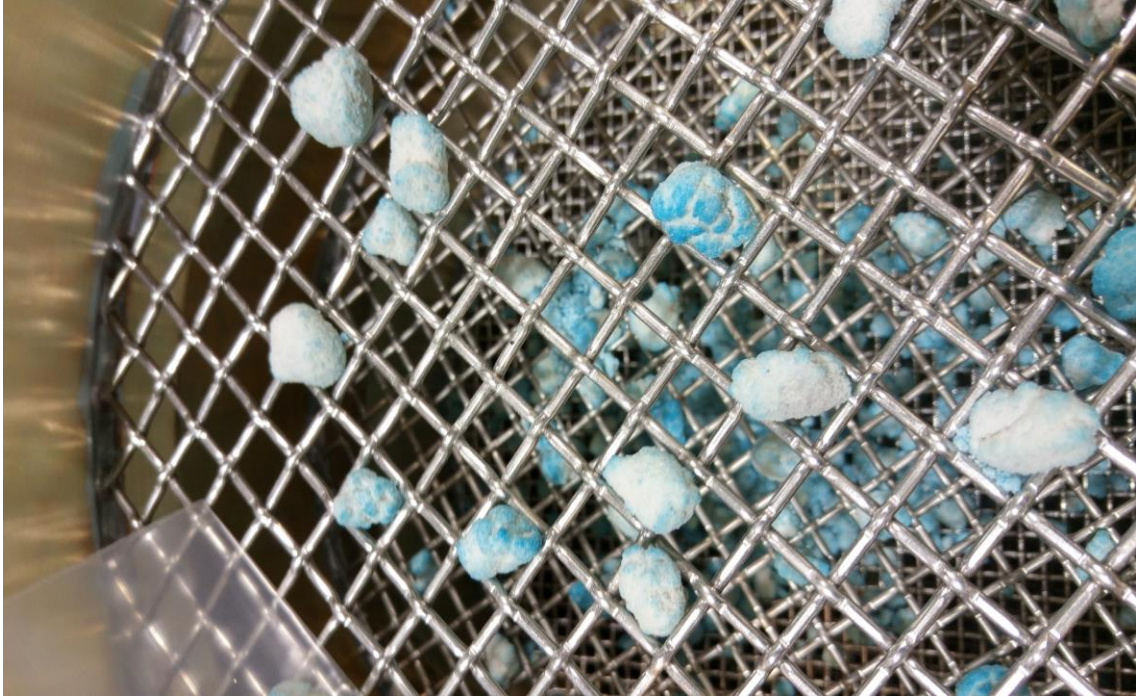
Figure 3-4: Agglomerates larger than 12500 \mu\text{m} collected from the bottom layer on a 12500 \mu\text{m} sieve at 0.60 m/s fluidization gas velocity
