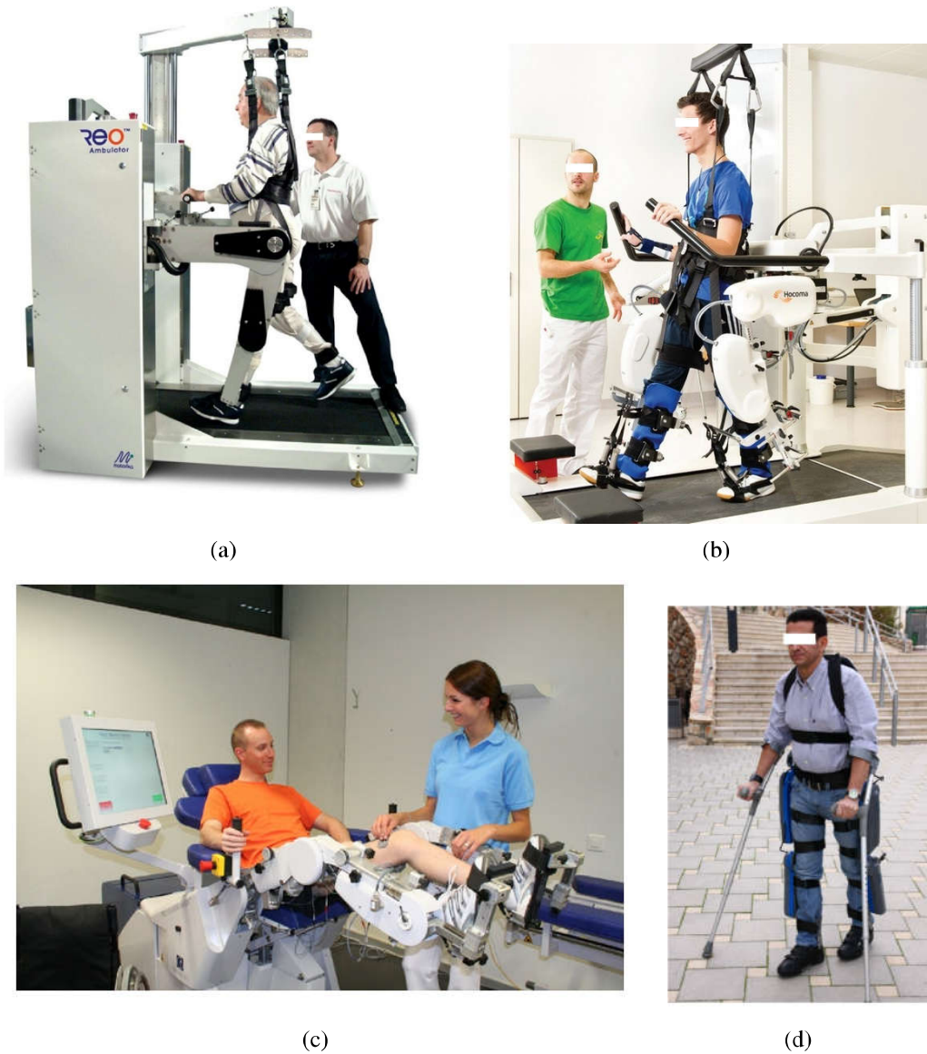
Figure 1.7: Exoskeleton type robots for gait training or stationary training on LE, (a) ReoAmbulator robotic system (Motorika Ltd.), (b) Lokomat system by Hocoma, (c) Motion-Maker (Swortec SA), and (d) ReWalk wearable system (ARGO Medical Technologies Ltd.) [15–18].
