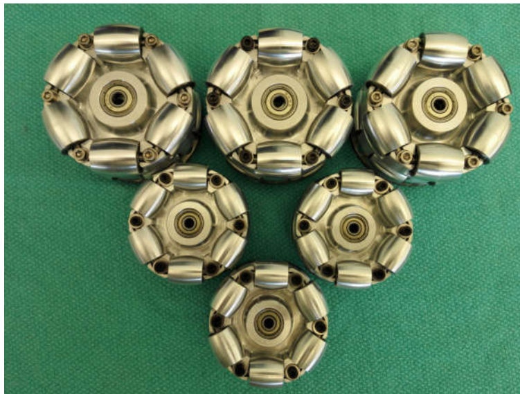
Figure 2.14: Manufactured Omni-wheels for mobile platform and orientations mechanism "A"
