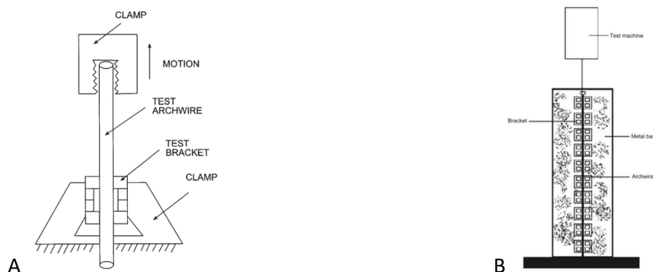
Figure 3: A. Set up of passive in vitro FR study 3 ; B. Passive in vitro FR study utilizing multiple aligned brackets. 6
