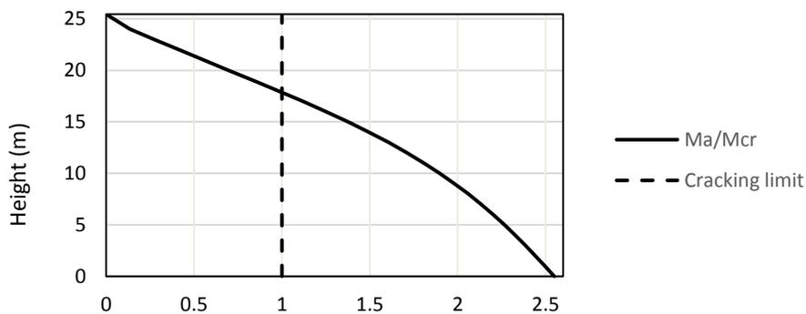
**Fig. 2-16.** Variation of  $(M_a/M_{cr})$  with the pole height
