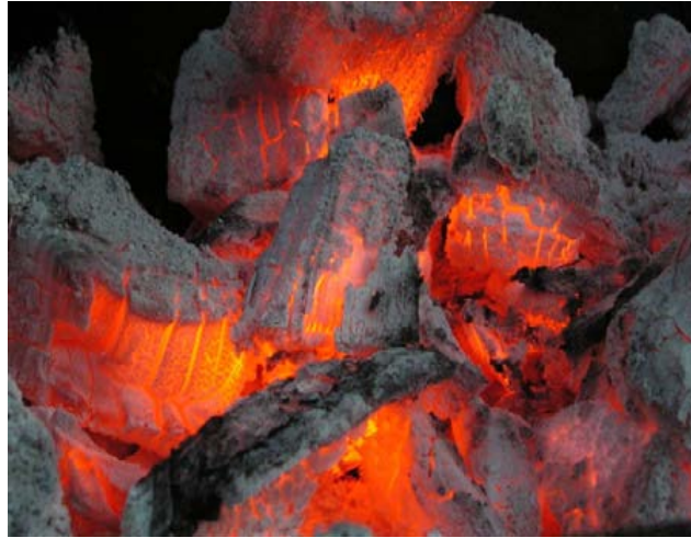
Figure 2-1. Smouldering combustion in char coal, where coal acts as both fuel and porous medium.
