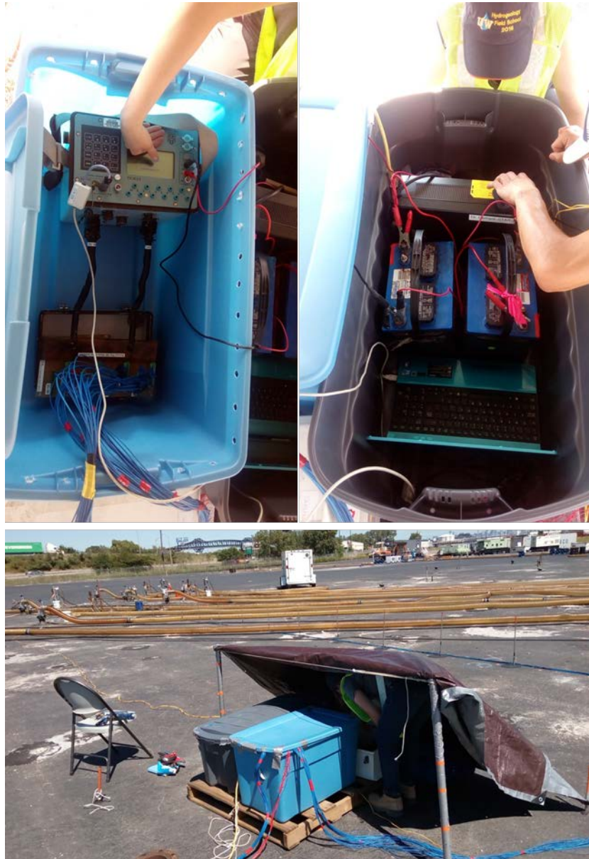
Figure B-4. (Top) Blue box contained the ERT equipment and switch box (right), while grey box contained the computer with battery support for the ERT equipment (left). (Bottom) Tarp was used to cover to protect from rain.
