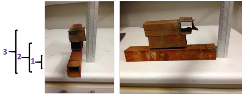
Figure E-3. Growing conductive target made of metal. Each image represents the addition of one metal bar perpendicular to the electrodes layout.
