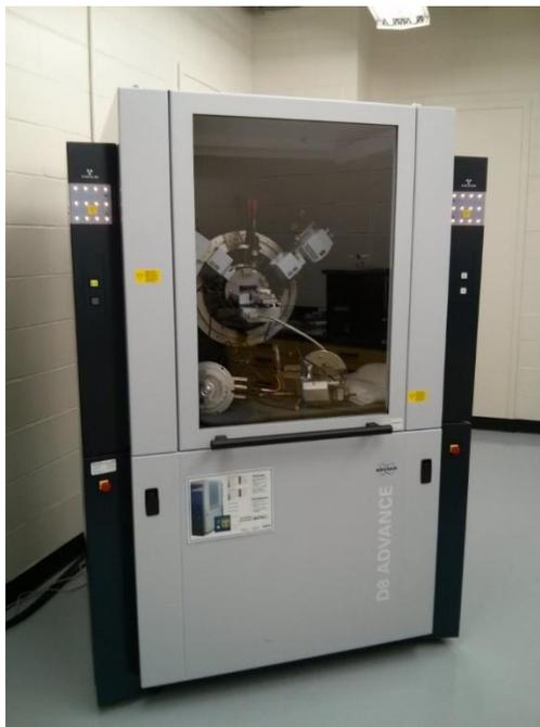
Figure 3-6 Digital photo of Bruker D8 Advance XRD machine.
