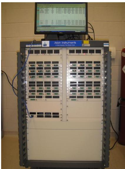
Figure 3-9 Digital photo of Arbin BT-2000 battery test station.
